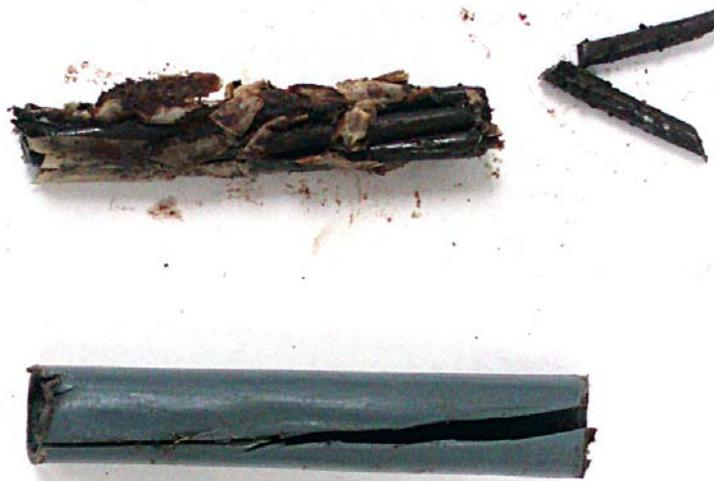
**Figure 27. Tendon A7 After Sheathing Removal**
