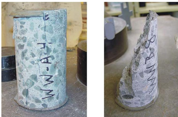
**Figure 16. Typical Fracture Patterns from Compressive Strength Tests**
