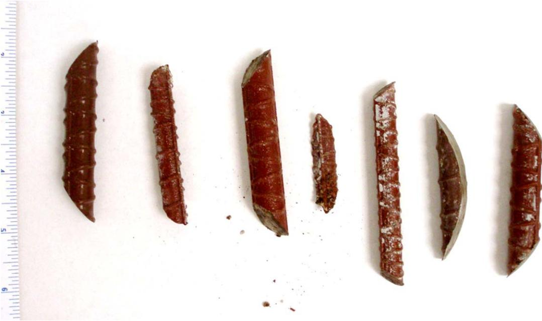
**Figure 22. Mild Reinforcement Bars from Precast Deck Slab Core Samples. The brown pigment color of the reinforcement coating should not be mistaken for corrosion product.**
