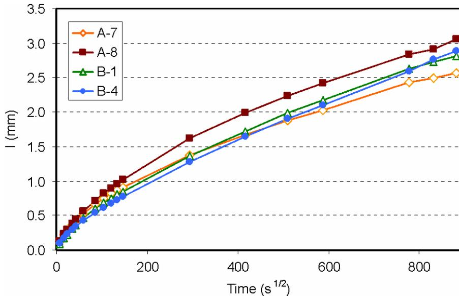
**Figure 19. Absorption Rates from ASTM C 1585-04**
