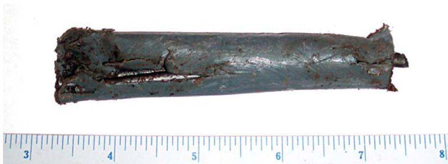
**Figure 23. Tendon A2 Prior to Sheathing Removal**
