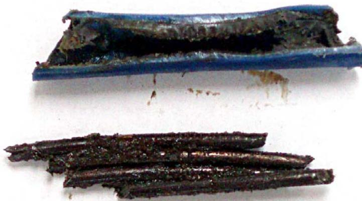
**Figure 28. Tendon B1 After Sheathing Removal**
