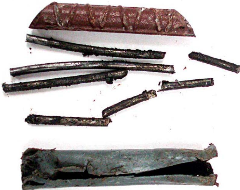
**Figure 26. Mild Reinforcement and Tendon A2 Strand and Casing After Sheathing Removal**
