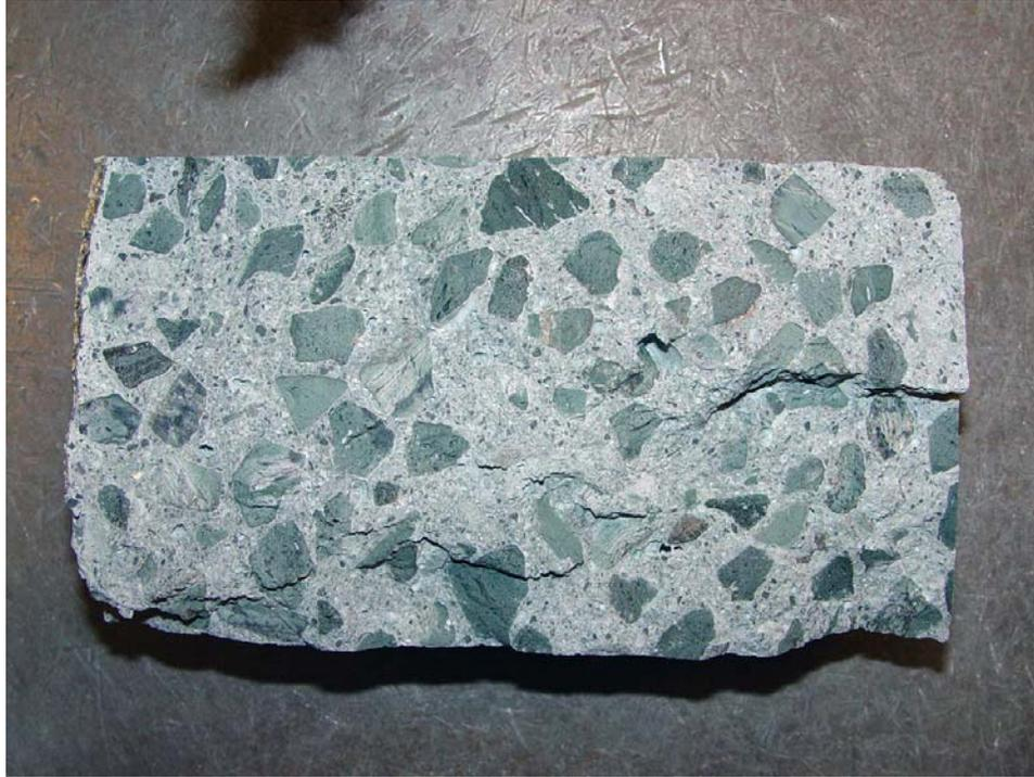
**Figure 17. Fracture Plane Passing Through Aggregate After Splitting Tensile Test**
