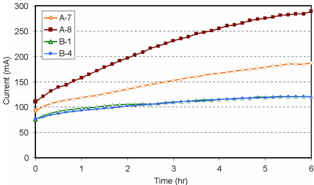
**Figure 20. Raw Data from Chloride Ion Penetration Test, ASTM C 1202-05**
