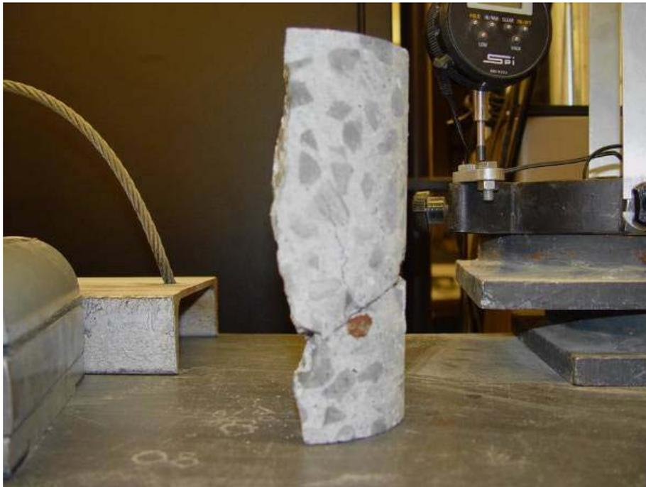
**Figure 18. Crack Forming Near Rebar After Splitting Tensile Test**
