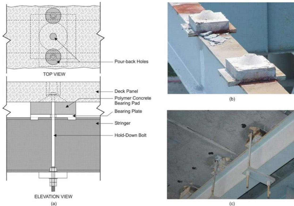
**Figure 3. Section of Precast Deck to Steel Girder Connection, Showing (a) Schematic of Entire Connection, (b) Cast Polymer Concrete Bearing Pad, and (c) Hold-Down Rods and Retainer Bar**
