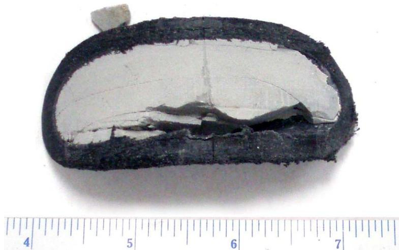
**Figure 32. Grout Sample in Duct**
