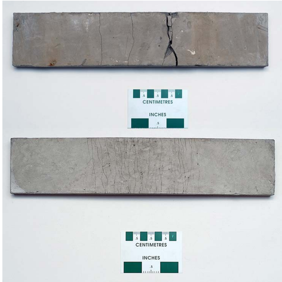
Figure 4. Cracks in Beam with Steel (SH) ( top ) and PVA Fibers ( bottom ). SH = twisted steel fiber, PVA = polyvinyl alcohol fiber.
