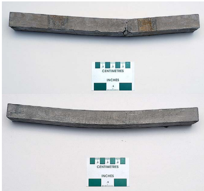
Figure 3. Large Deflections in Beam with Steel (SH) (top) and PVA Fibers (bottom). SH = twisted steel fiber, PVA = polyvinyl alcohol fiber.
