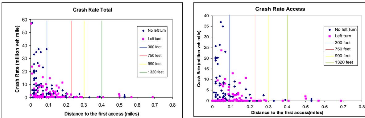
Figure 21. Crash Rate as a Function of the Presence of a Left Turn Storage Lane
