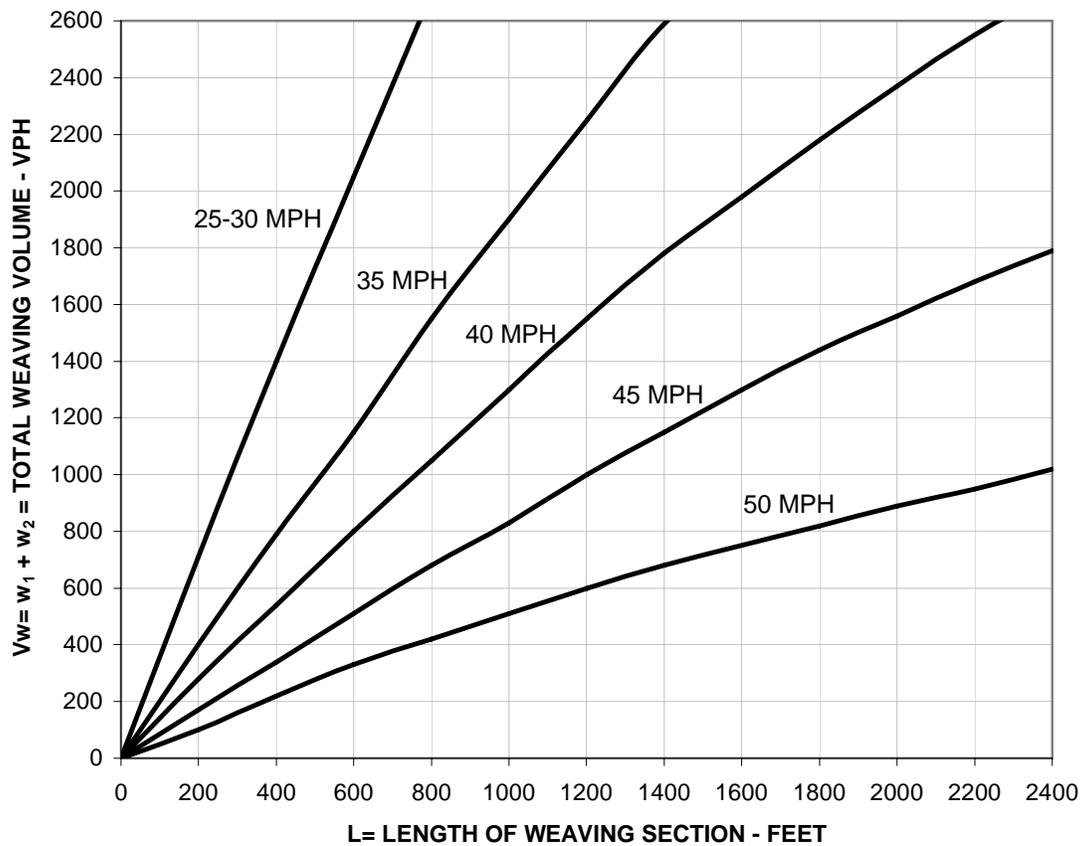
**Figure 2. Analysis of Service Road Weaving Conditions (Layton, 1996)**
