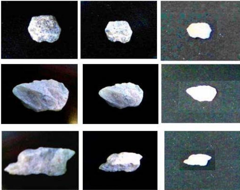
Figure 13. Aggregate pictures taken at (a) 2 in (5 cm), (b) 3 in (7.5 cm), and 10 in (25 cm)
