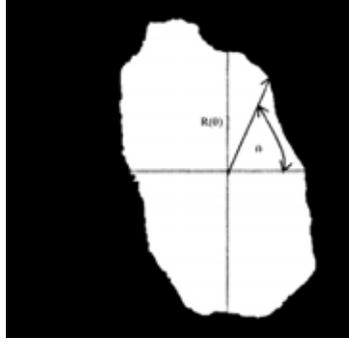
**Figure 4. Illustration of Fourier boundary representation (Wang et al. 2005)**
