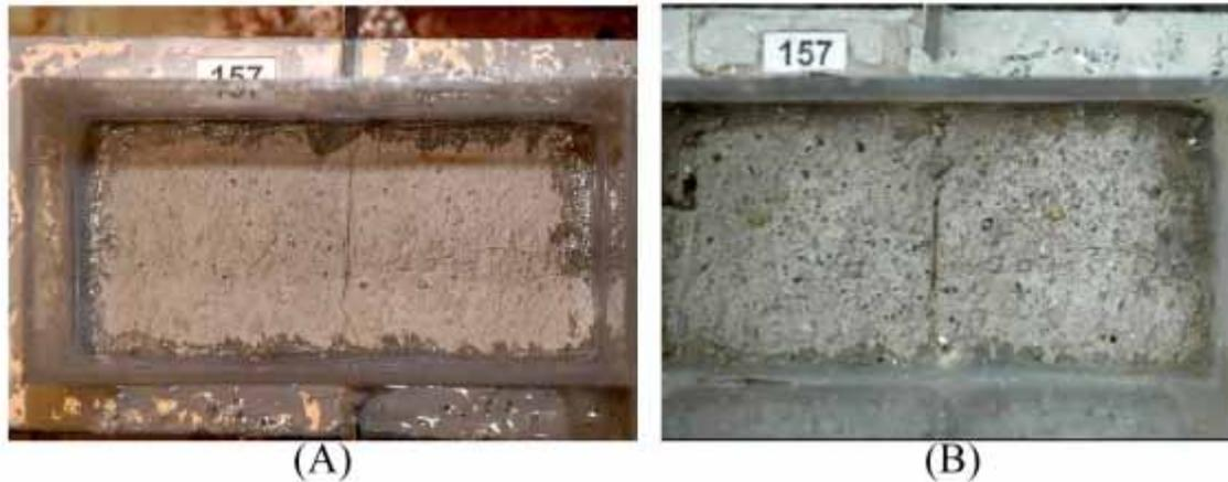
**Figure 16. Typical view of specimen (A) before testing and (B) after testing, showing no outward signs of corrosion.**
