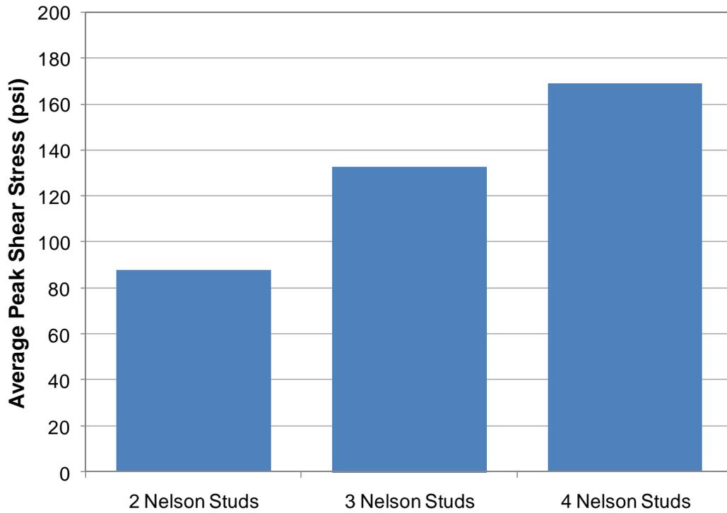
Figure 53. Average Peak Shear Stresses for Headed Shear Stud Tests.
