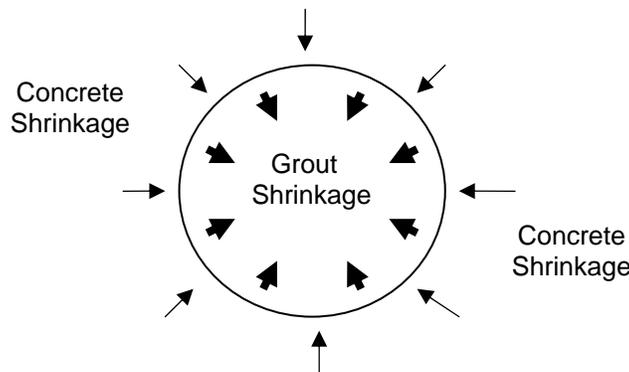
**Figure 30. Differential Concrete and Grout Shrinkage at Shear Pocket Interface**
