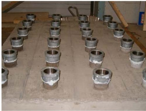
**Figure 20. Steel Caps Glued to Grout Discs with PC-11<sup>®</sup> White Epoxy Paste**
