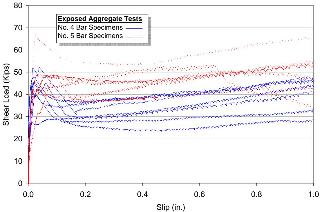
**Figure 52. Load versus Slip for Exposed Aggregate Tests**
