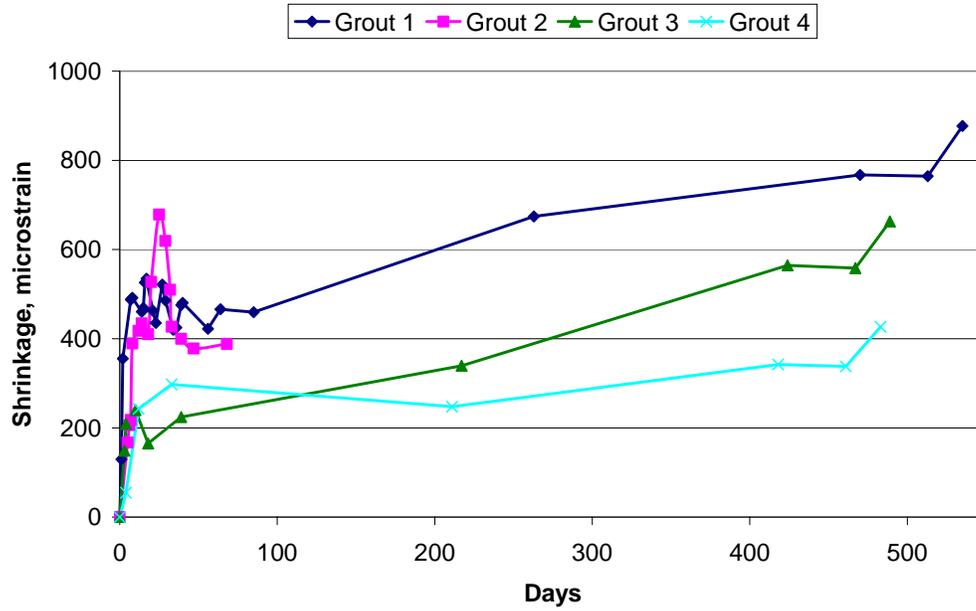
Figure 31. Differential Shrinkage of Concrete and Neat Grouts
