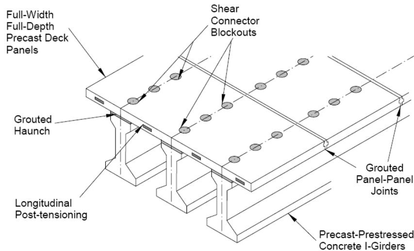
**Figure 1. Representation of Bridge Deck Panel System**
