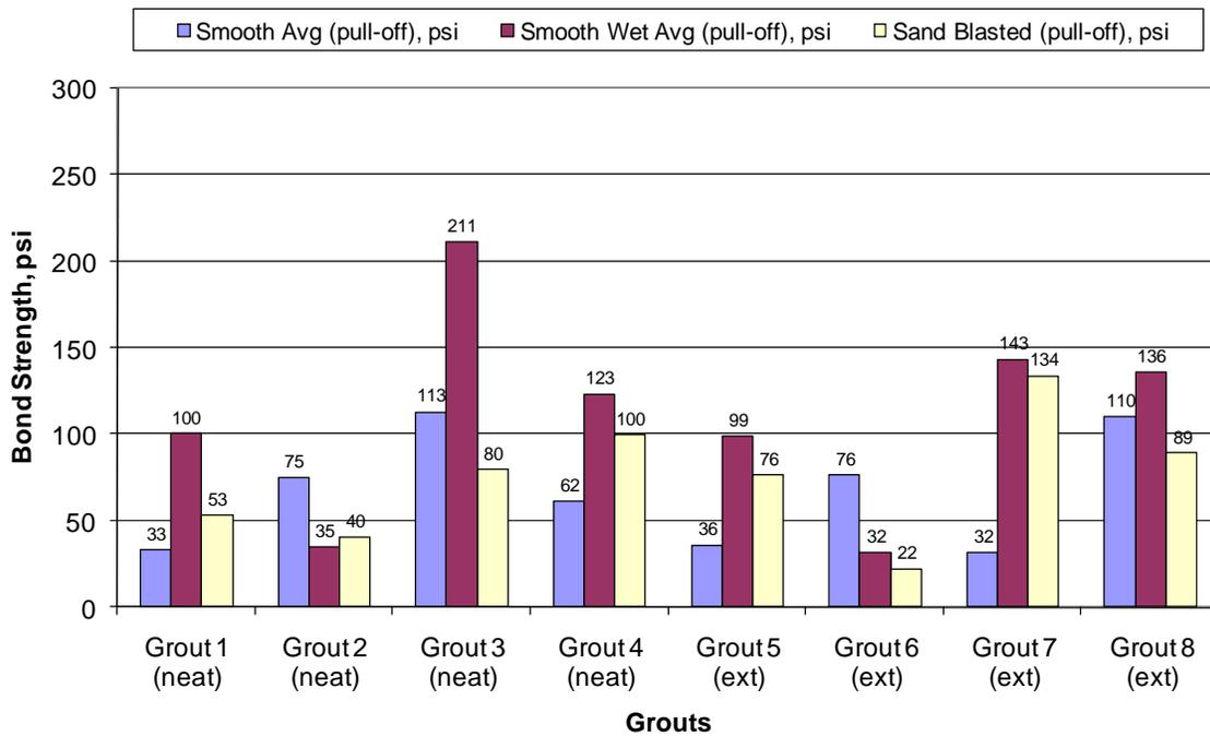
Figure 45. Comparison of All Pull-off Tests Results
