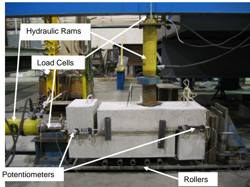
**Figure 17. Push-Off Test Setup**
