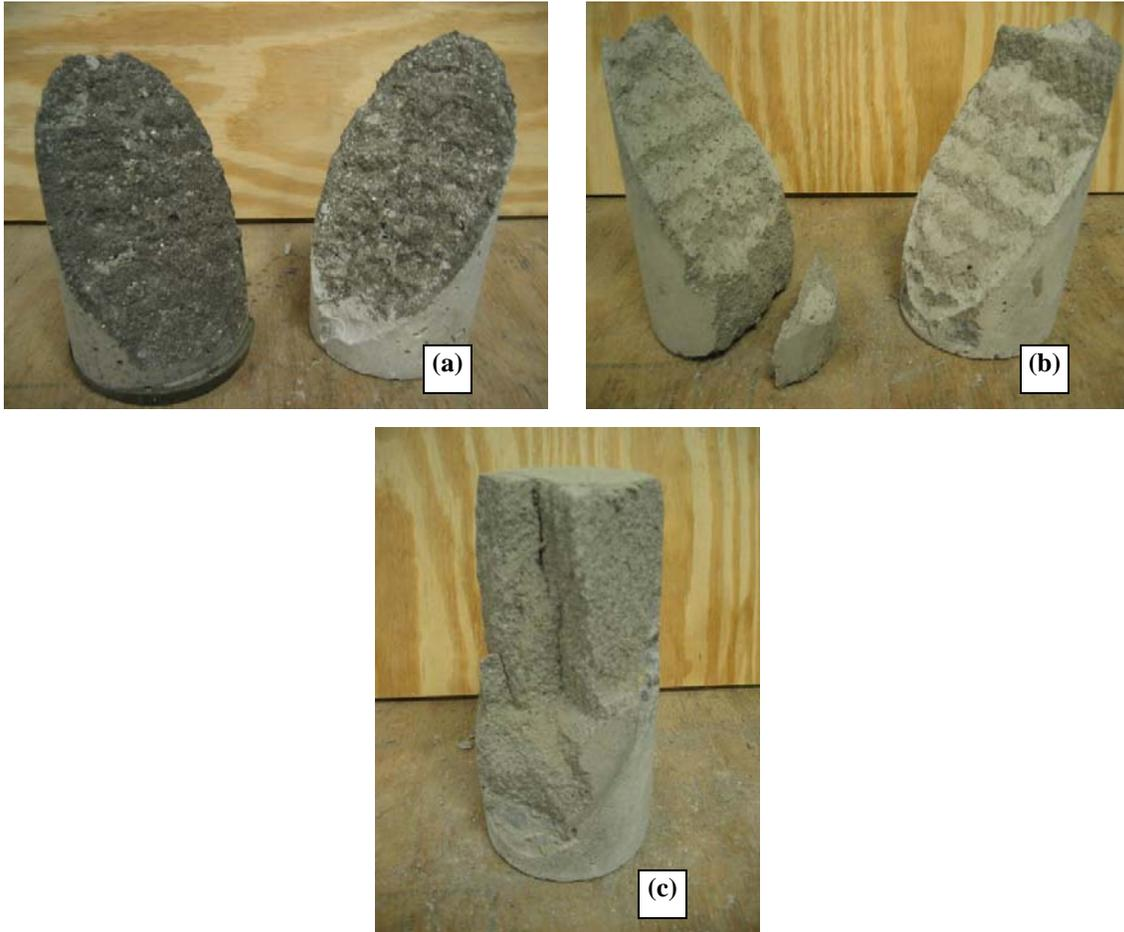
**Figure 38. Slant Shear Cylinder Failure Modes**
