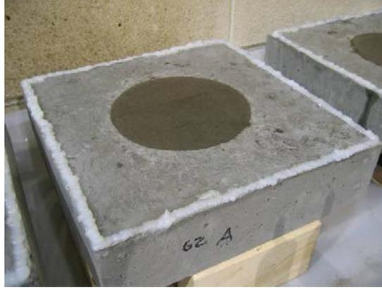
**Figure 4. Shear Pocket Specimen with Water Ponding**
