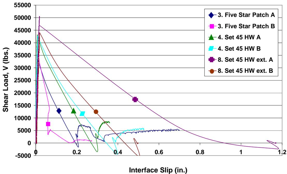
Figure 40. Push-Off Test Shear Load vs. Interface Slip
