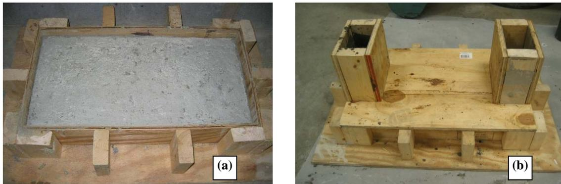
**Figure 6. Haunch Flow Mockup Before (a) and After (b) Placement of Cover**
