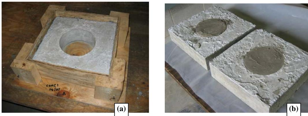
**Figure 3. Shear Pocket Specimen Before (a) and After (b) Filling with Grout**
