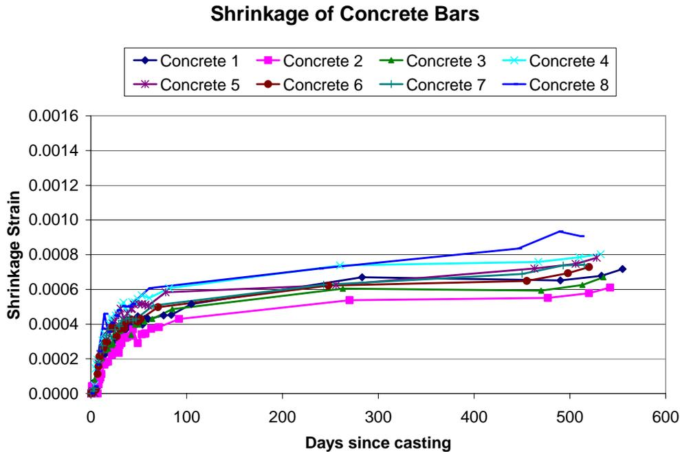
Figure 27. Concrete shrinkage
