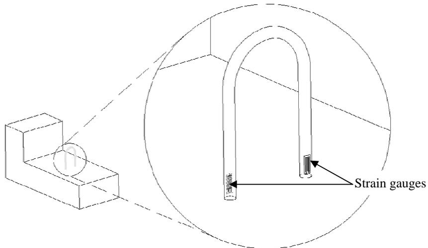
**Figure 24. Strain Gage Placement**
