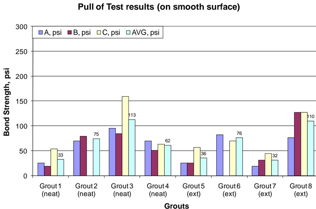
**Figure 42. Results from Pull-off Tests Performed on Smooth Dry Surface**
