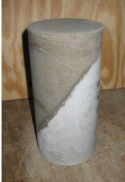
**Figure 11. Completed Slant Shear Cylinder**
