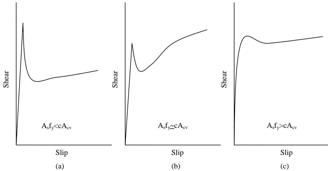
**Figure 46. Typical Load vs. Slip Plots**
