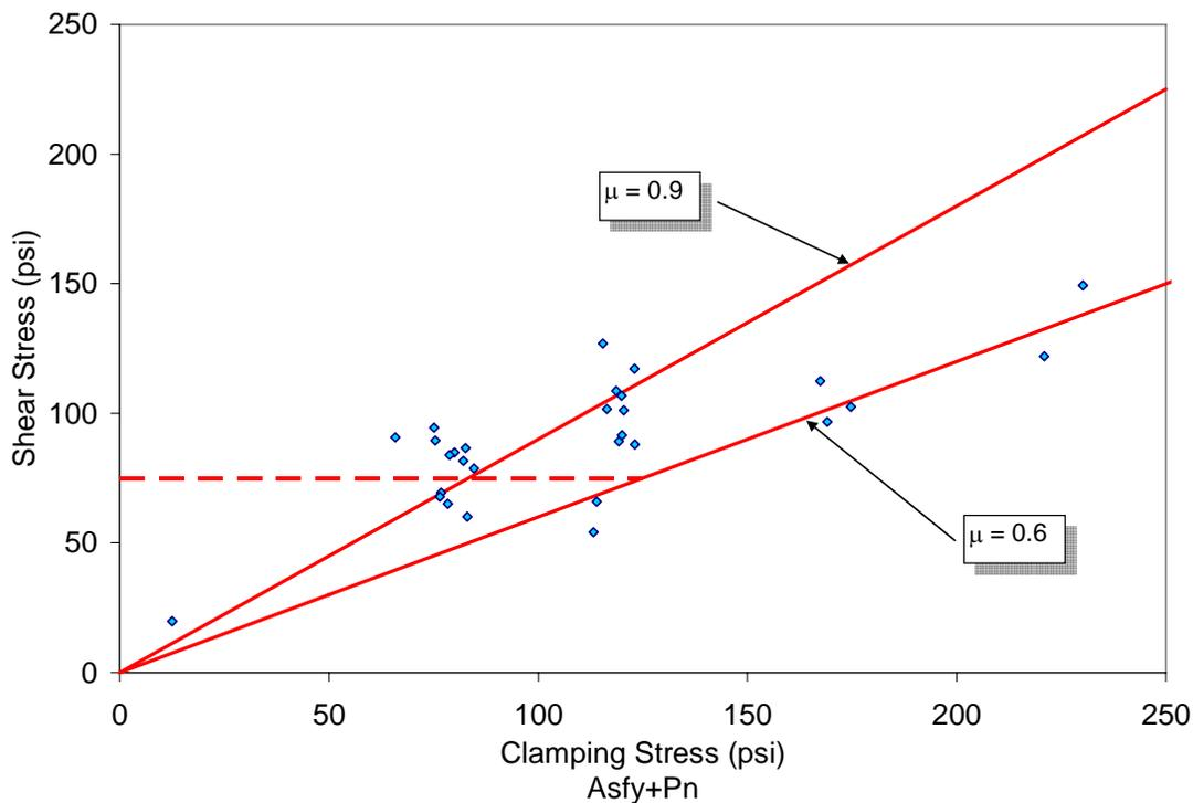
**Figure 61. Post Peak Results with Proposed Equations**
