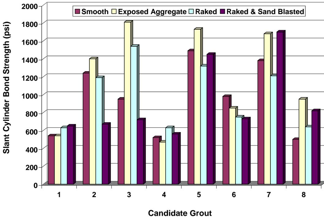
**Figure 39. Slant Cylinder Bond Strength with Varying Concrete Surface Preparations**
