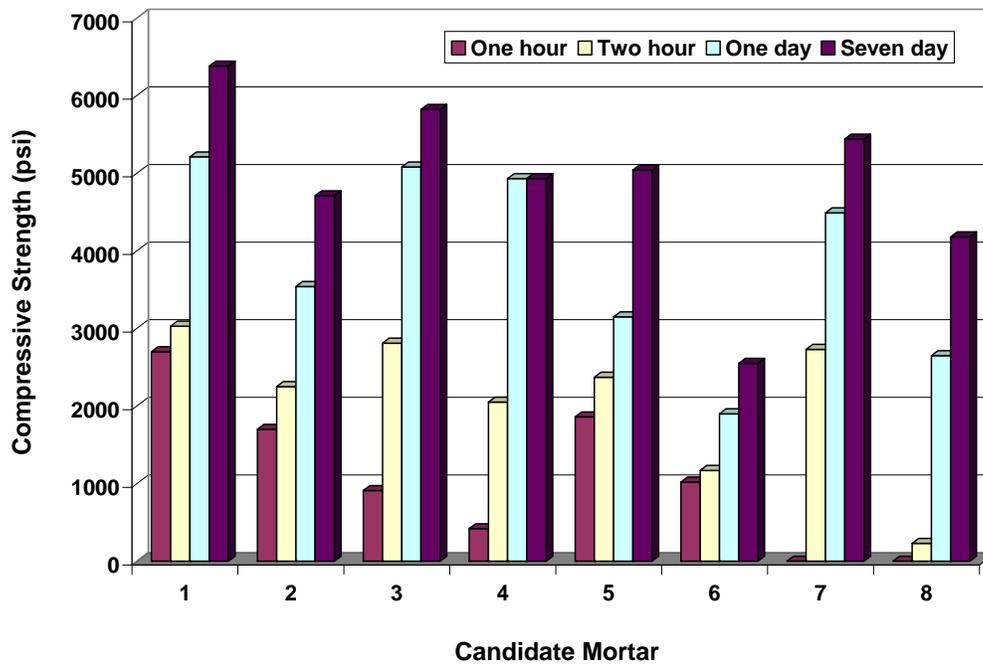
**Figure 25. Compressive Strengths per ASTM C 109**
