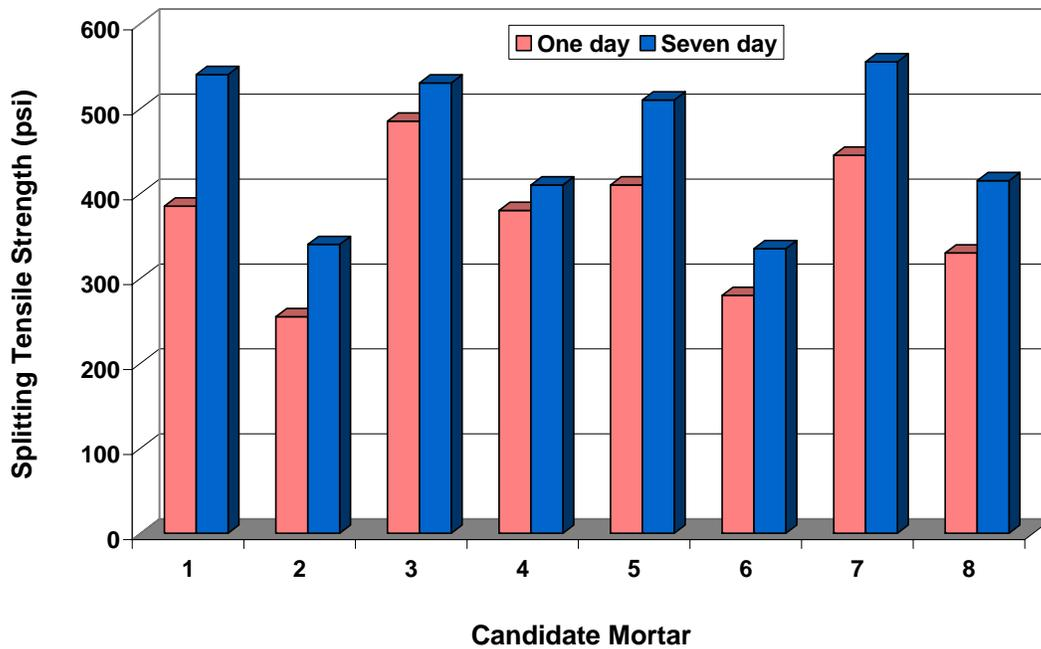
**Figure 26. Splitting Tensile Strengths per ASTM C 496**
