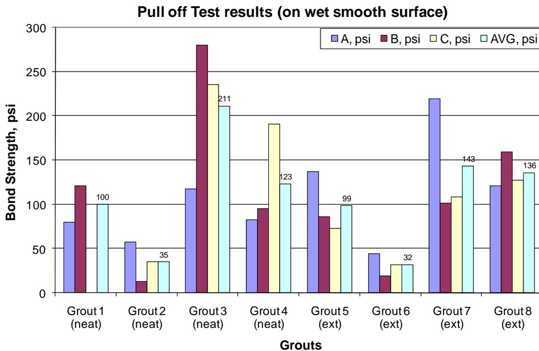
**Figure 43. Results from Pull-off Tests Performed on Smooth Saturated Surface Dry Surface**
