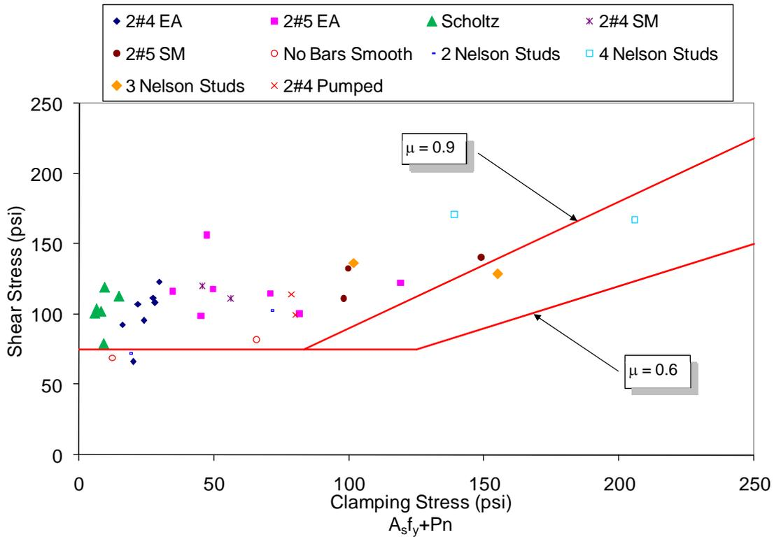
**Figure 60. Peak Shear Stress Results with Proposed Equations**
