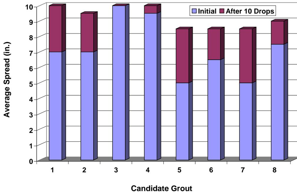
Figure 35. Truncated Flow Cone Spread Values per ASTM C 1437
