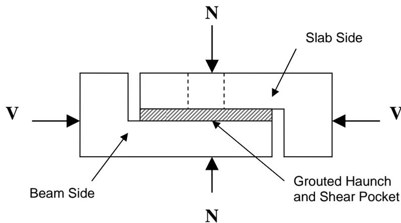
**Figure 12. Typical Push-Off Test Setup**
