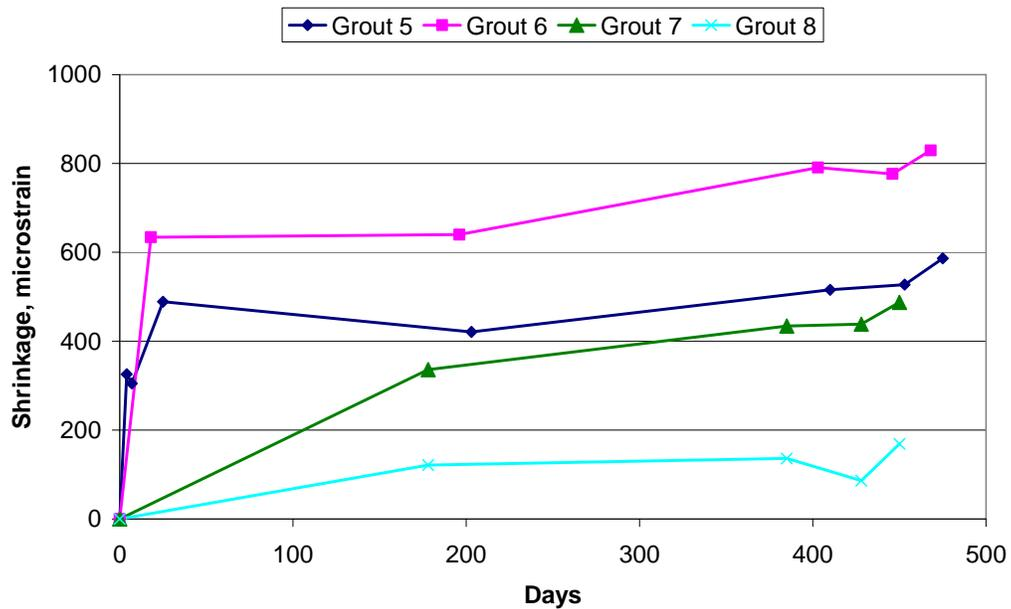
Figure 32. Differential Shrinkage of Concrete and Extended Grouts
