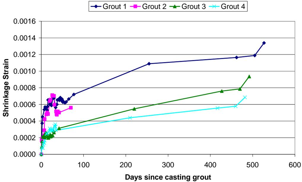
**Figure 28. Shrinkage of Neat Grouts per ASTM C 157**
