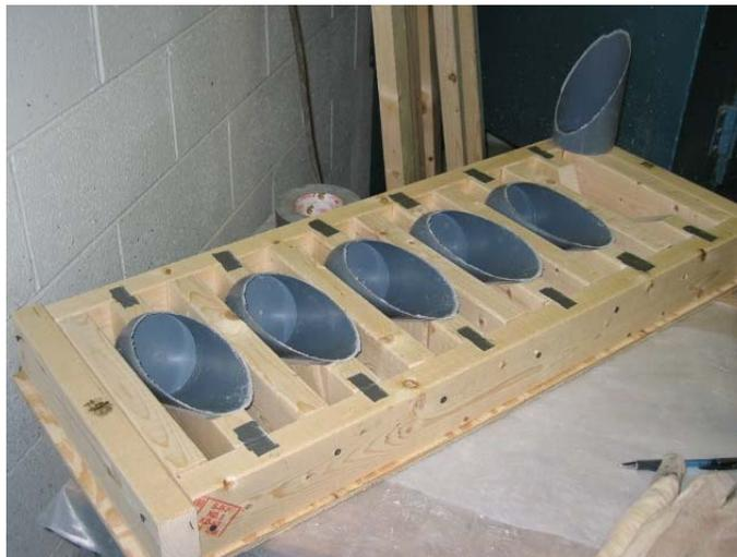
**Figure 9. Sliced 4 in. x 8 in. Cylinders for Slant Cylinder Tests**
