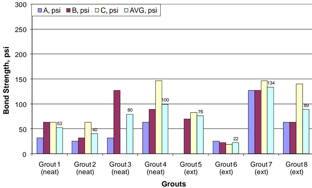
Figure 44. Results from Pull-off Tests Performed on Sand-blasted Smooth Wet Surface
