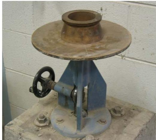
**Figure 5. Truncated Flow Cone and Drop Table**
