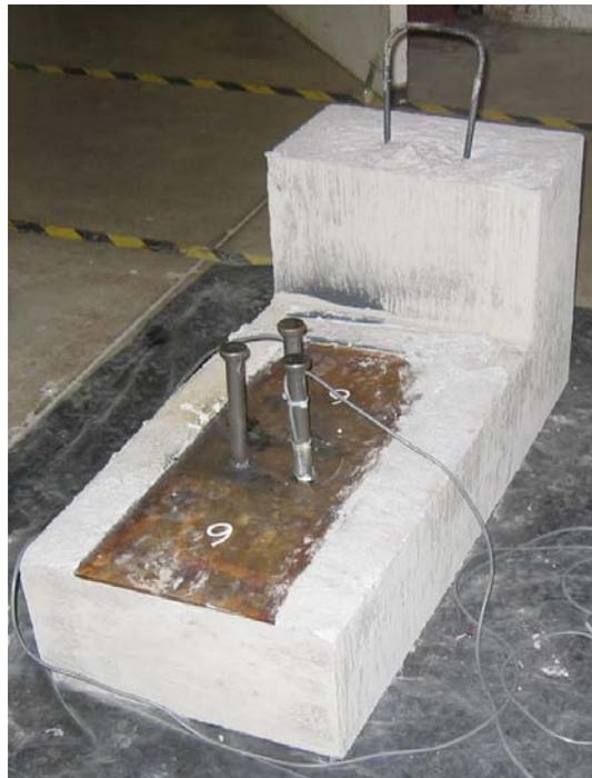
**Figure 22. Headed Shear Stud Specimen**
