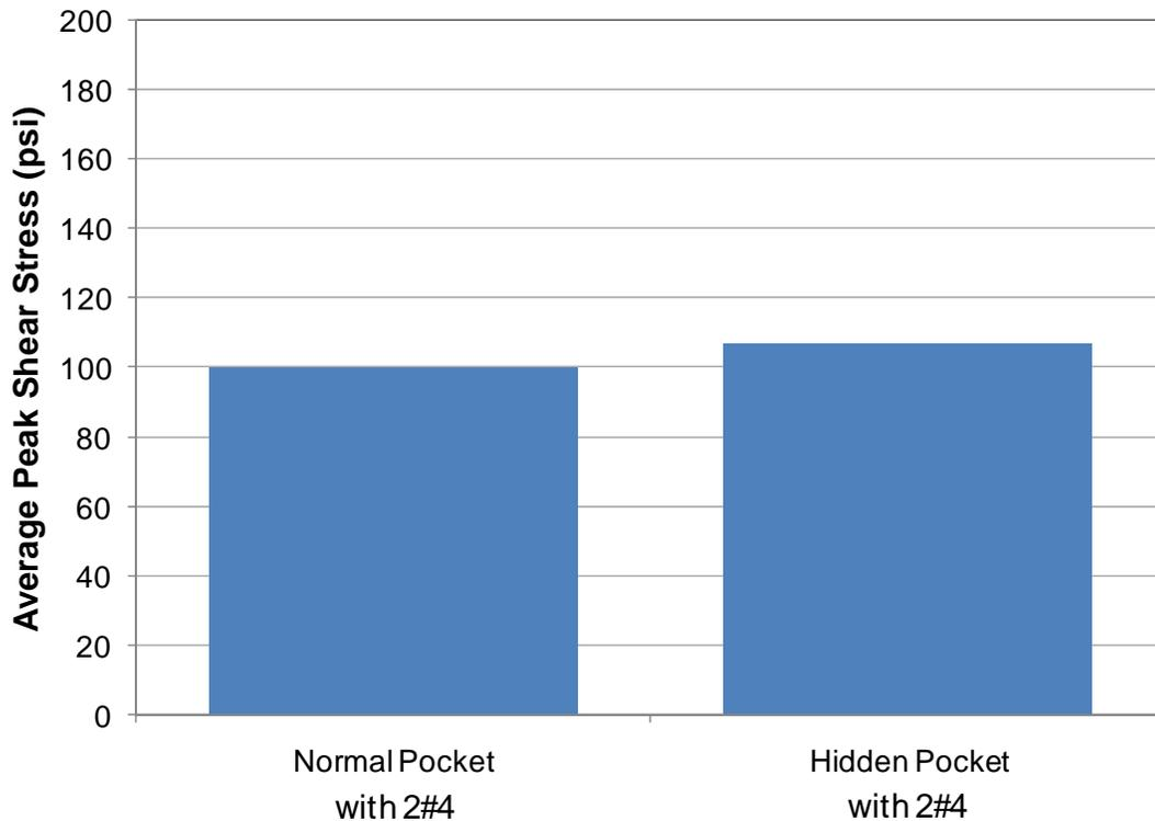
Figure 55. Normal Pocket versus Hidden Pocket Average Peak Shear Stress
