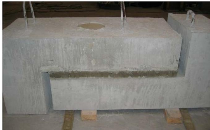
**Figure 16. Complete Push-Off Specimen with Grouted Interface**
