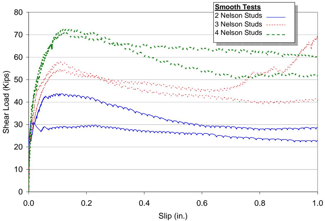
Figure 54. Load versus Slip for Headed Shear Stud Tests
