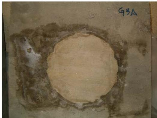
**Figure 33. Five Star® Patch Neat (3) Shear Pocket Showing Water Leaking at 12 Months**
