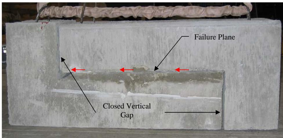
**Figure 47. Push-Off Specimen after Failure**
