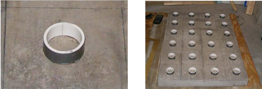
**Figure 19. PVC Molds for a Grout Disc to be Used in Pull-off Tests Glued to Concrete Slab**
