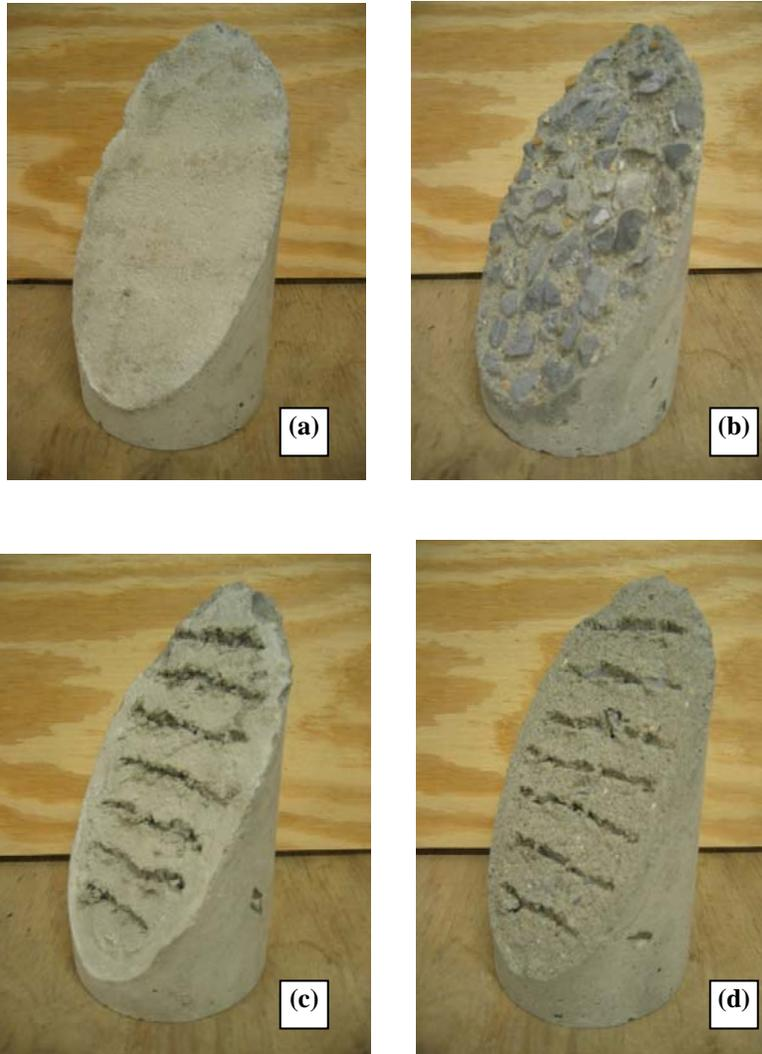
**Figure 10. Slant Cylinder Concrete Surface Preparations:
