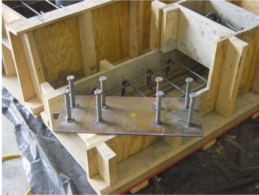
Figure 50. Plate to be embedded in top of beam side specimen
