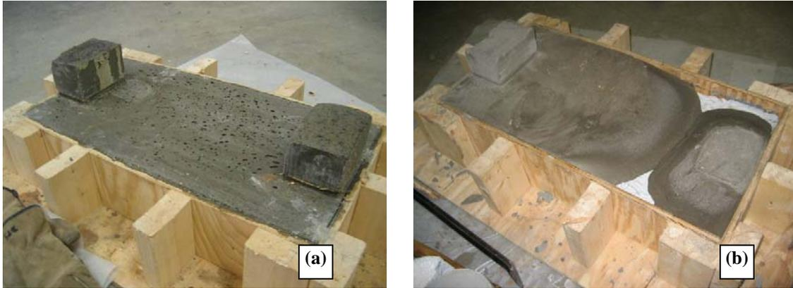
**Figure 7. Good (a) and Poor (b) Grout Flow Through Haunch Mockup**
