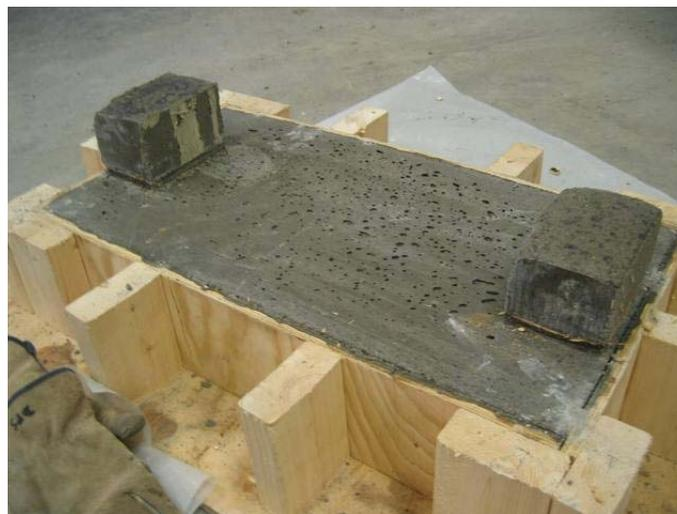
Figure 37. Set<sup>®</sup> 45 Hot Weather (4) Flow Through Haunch Mockup
