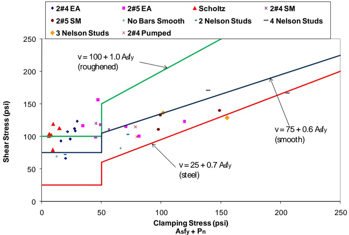
Figure 59. Peak Shear Stress vs. Clamping Stress
