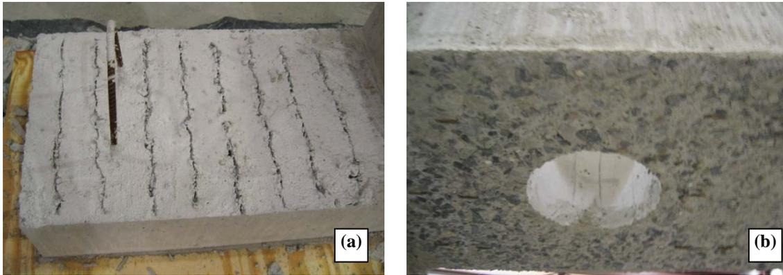
**Figure 15. Beam Side (a) and Slab Side (b) Push-Off Specimen Surface Preparation**
