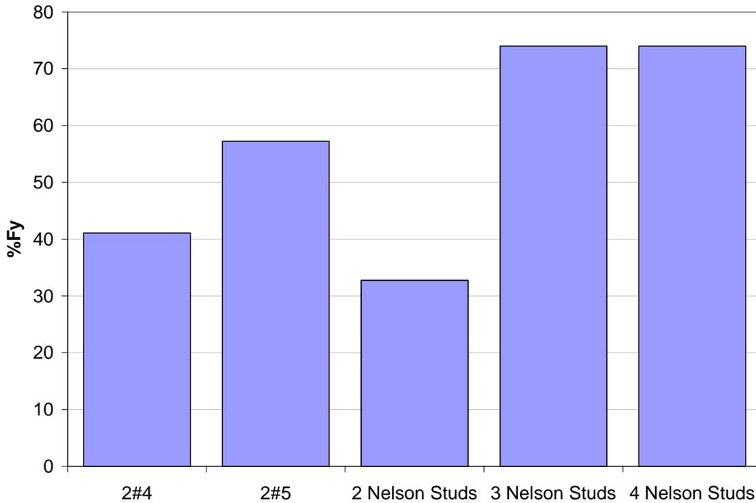
**Figure 56. Percent of Yield Stress in Shear Connectors at Peak Load**
