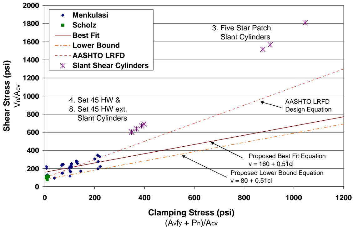
**Figure 41. Shear Stress vs. Clamping Stress with Slant Shear Cylinders**
