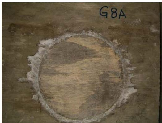
**Figure 34. Set® 45 HW Extended (8) Showing Dampness and Efflorescence at 12 Months**
