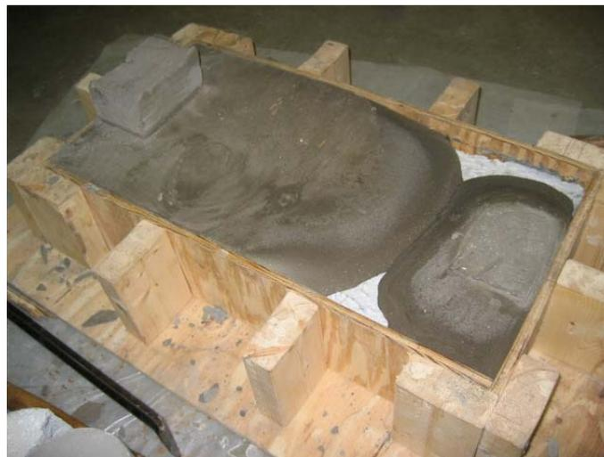
Figure 36. ThoRoc® 10-60 (1) Flow Through Haunch Mockup
