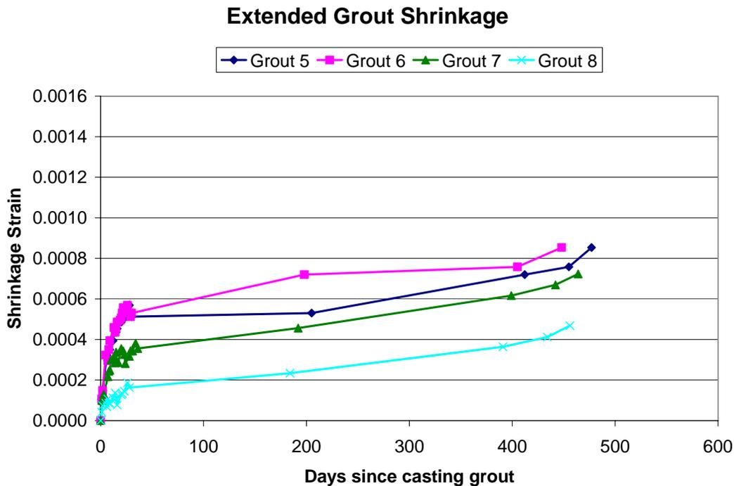
**Figure 29. Shrinkage of Extended Grouts per ASTM C 157**
