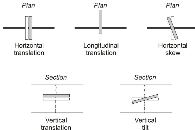
**Figure 1. Categories of Dowel Misalignments<sup>1,7</sup>**
