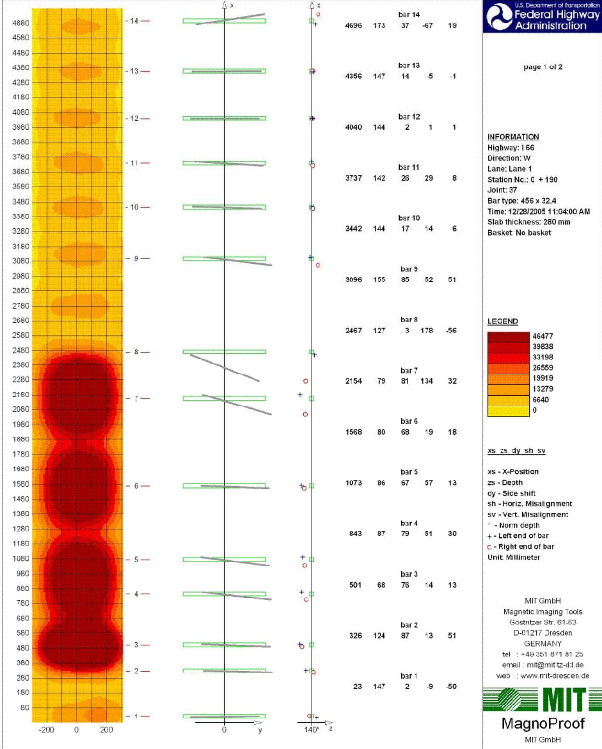
Figure 10. Signal Looping for Joint 37 on I-66
