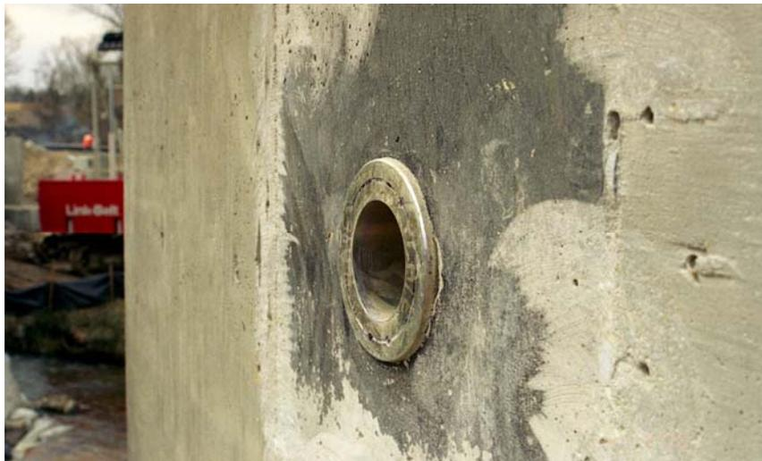
**Figure 12. Load Cell at Abutment B**
