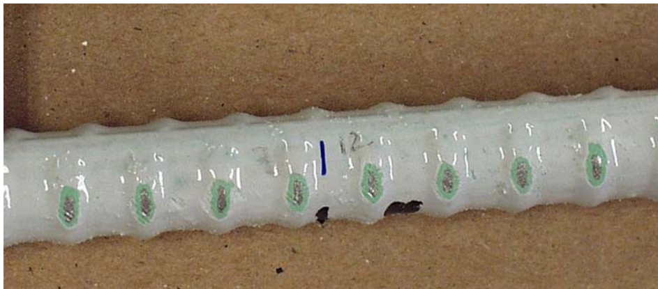
Figure 4. No. 5 Epoxy-Coated Bar Damaged Prior to Placement in Type I Concrete Test Beam. The black marking along the bar but below the damaged coating is from a permanent marker and is not part of the coating damage.
