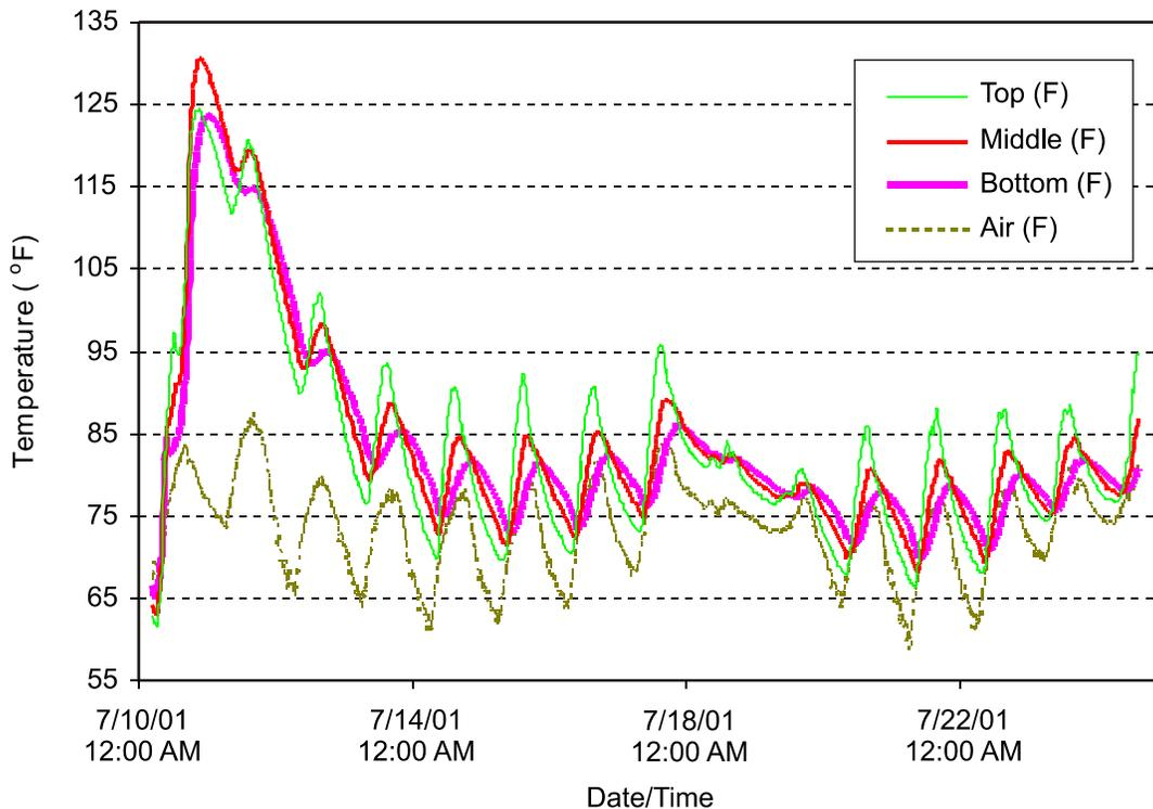
**Figure 4. Temperatures at Varying Depths of Deck Concrete**
