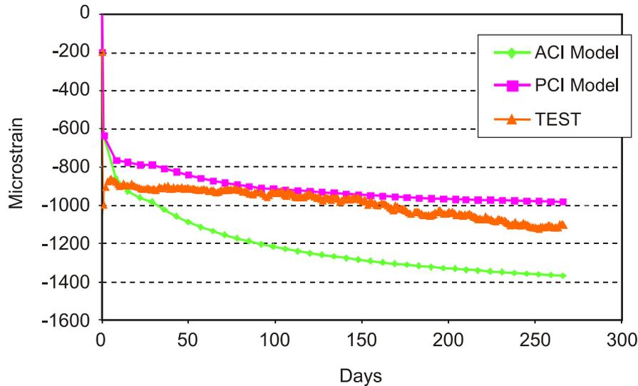
**Figure 3. Concrete Strains Over Time**
