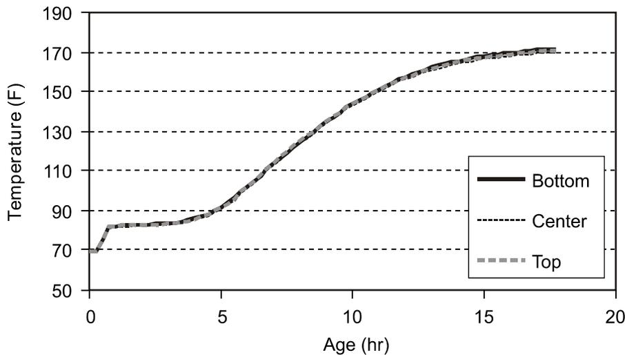
**Figure 1. Temperature Data for Bridge Beam 1**
