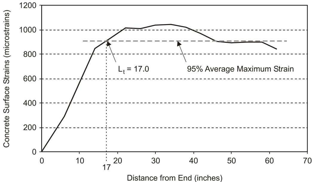
**Figure 2. Average Strain Data Profile for Type IV Beams**
