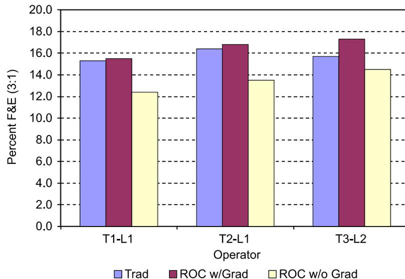
**Figure 6. Average F&E Versus Reduction Procedure. Trad. = Traditional method; ROC w/Grad = ROCLOG software using full gradation results for aggregate source; ROC w/o Grad = ROCLOG estimate only.**
