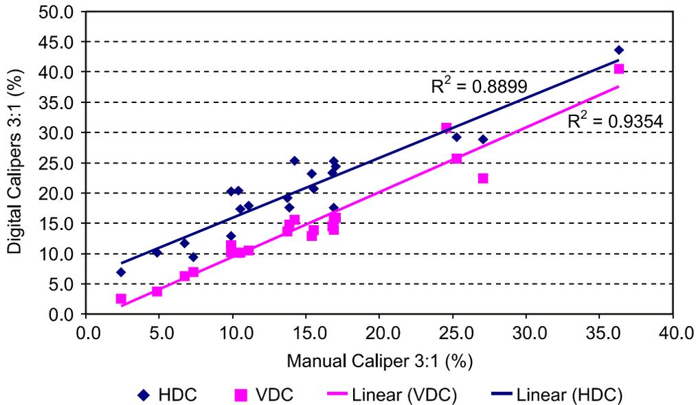
**Figure 3. Digital Caliper Results as Function of Manual Caliper (Technician No. 1, 3 devices, 22 sources)**
