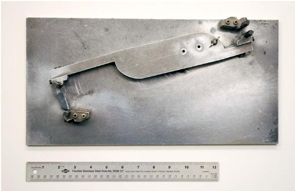
**Figure 1. Mechanical Proportional Caliper**
