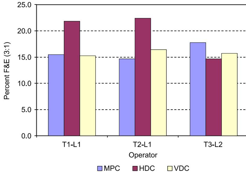
**Figure 4. Average F&E Particle Content (3 technicians, 3 devices, 10 sources). MPC = manual proportional caliper; HDC = horizontal digital caliper; VDC = vertical digital caliper; T1-L1 = Technician 1-laboratory 1, etc.**
