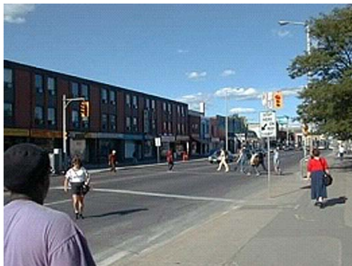
Figure B17. Pedestrian-Actuated Mid-block Signal. From www.pedbikeimages.org / ITE Pedestrian Bicycle Council. Reprinted with permission.
