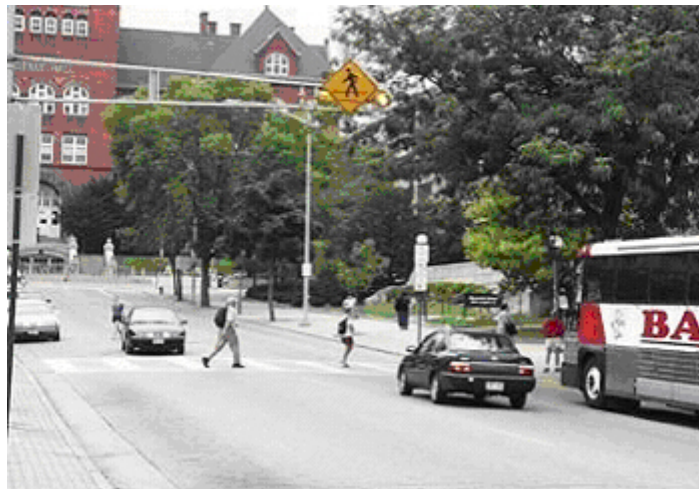
Figure B14. Overhead Sign with Flashing Beacons. From www.pedbikeimages.org/ ITE Pedestrian Bicycle Council. Reprinted with permission.
