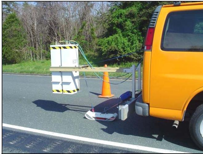
**Figure 1. Van used for GPR data collection**
