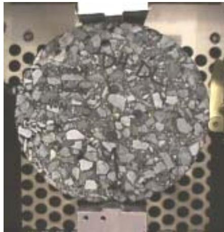
**Figure 3. Specimen split after an IDT strength test**
