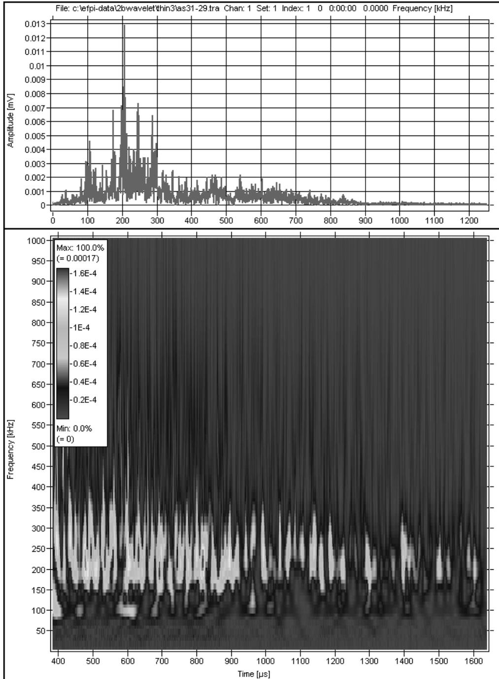
Figure 23. (top) Fast-Fourier Transform (FFT) amplitude versus frequency plot for an AE signal detected during the initial loading of a thin HPS70W specimen, (bottom) Wavelet Transform, frequency versus time.
