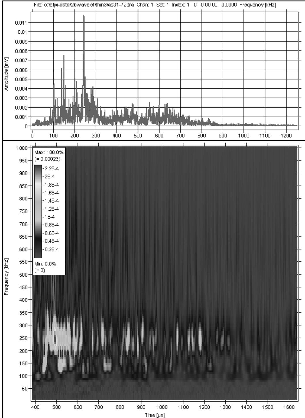
Figure 25. (top) Fast-Fourier Transform (FFT) amplitude versus frequency plot for an AE signal detected during the initial loading of a thin HPS70W specimen 3, (bottom) Wavelet Transform, frequency versus time.
