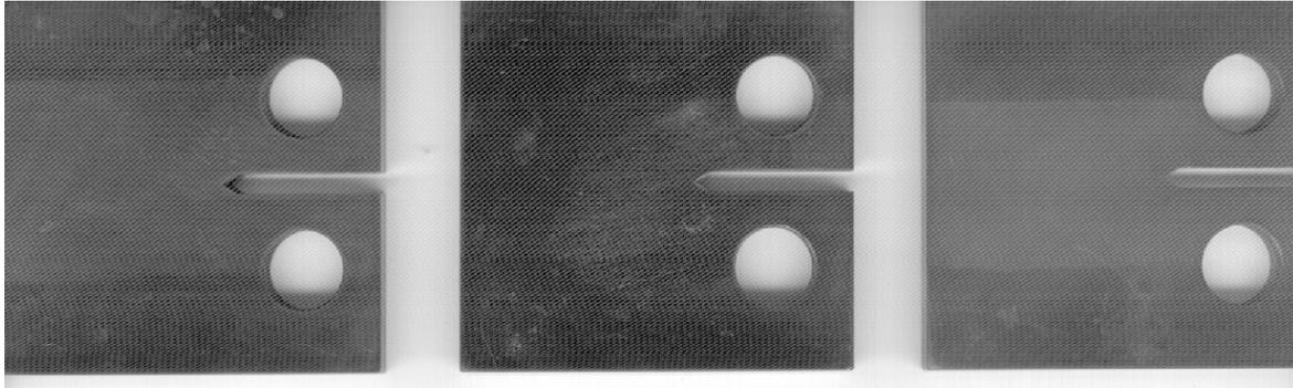
Figure 19. Images of three thin HPS70W [due to limited material no lip was included] where the central welded region is visible due to slight difference in coloration of the surface.
