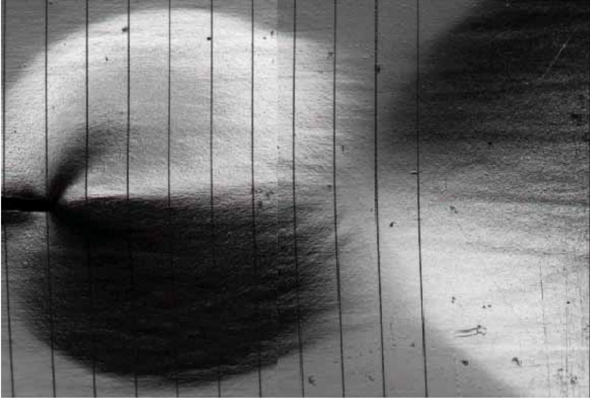
Figure 9b. Image of the plastic zone surrounding the crack for an HPS 70W specimen following the twelfth overload shown at the same magnification as 9a); two images have been overlapped to show the entire zone at this magnification.
