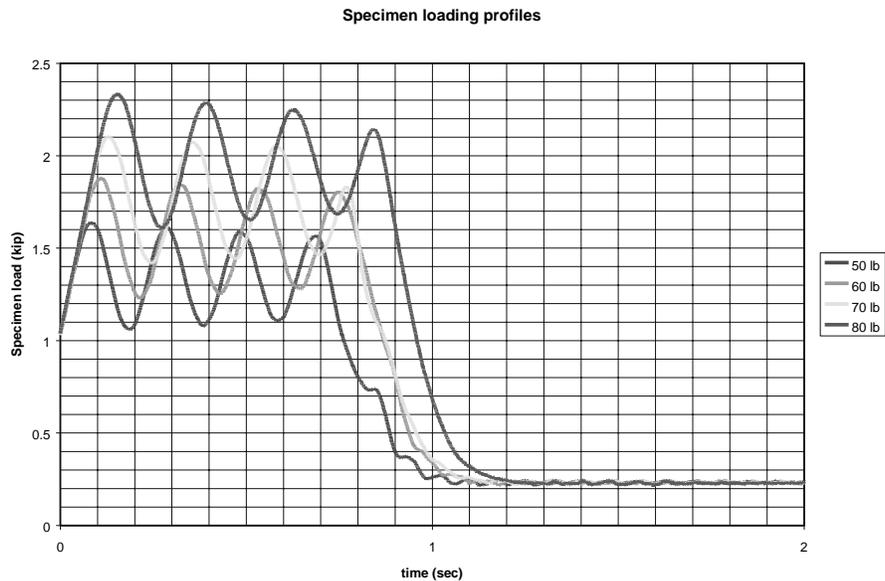
Figure 2. Plots of the load variation for loads on the weight pan of 50, 60, 70, and 80 lb.
