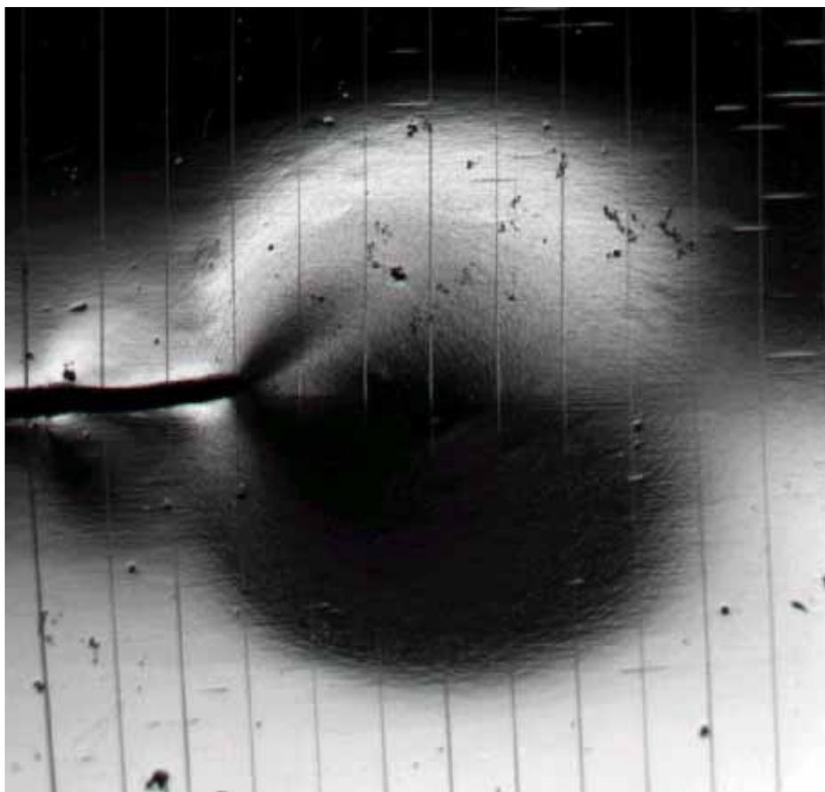
Figure 10. Image of the plastic zone for an A588 specimen following the eleventh overload.
