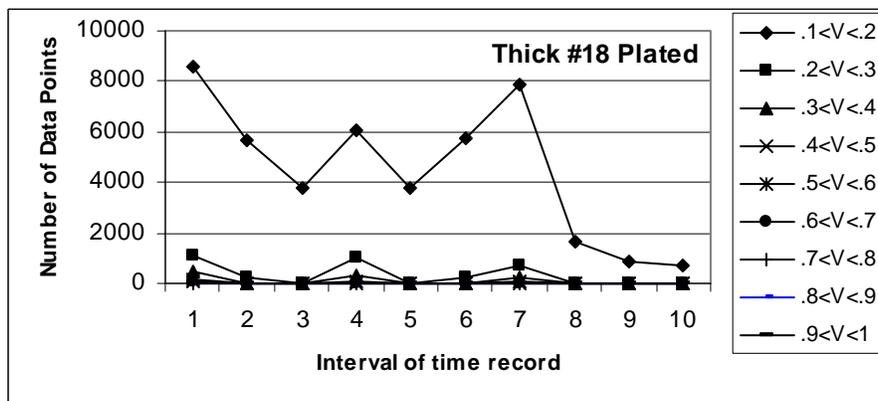
Figure 18. Family of curves showing the distribution of amplitudes over the loading period for specimen 5
