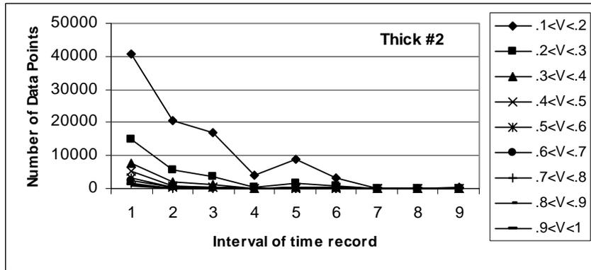
Figure 15. Family of curves showing the distribution of amplitudes over the loading period for thick specimen 2.
