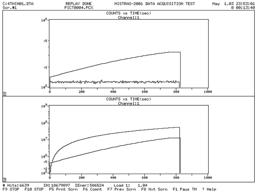
Figure 21a. Plots showing 1) the AE counts versus time and 2) the summation of AE counts versus time during the initial loading. Superimposed on both plots is the load versus time, where full scale represents 2000 lb.
