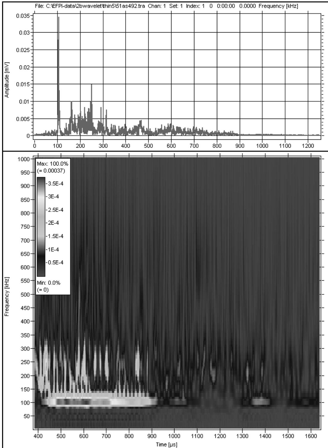
Figure 26. (top) Fast-Fourier Transform (FFT) amplitude versus frequency plot for an AE signal detected during the initial loading of a thin HPS70W specimen 5, (bottom) Wavelet Transform, frequency versus time
