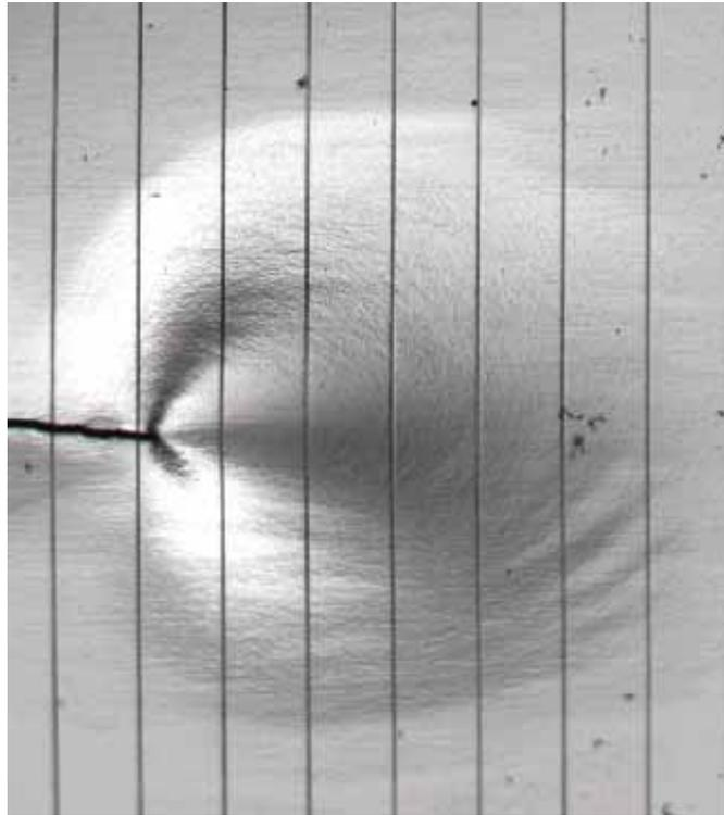
Figure 9a). Image of the plastic zone surrounding the crack for an HPS 70W specimen following the eleventh overload.
