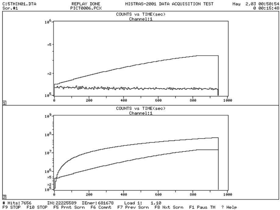
Figure 22a. Plots showing 1) the AE counts versus time and 2) the summation of AE counts versus time during the initial loading. Superimposed on both plots is the load versus time, where full scale represents 2000 lb.
