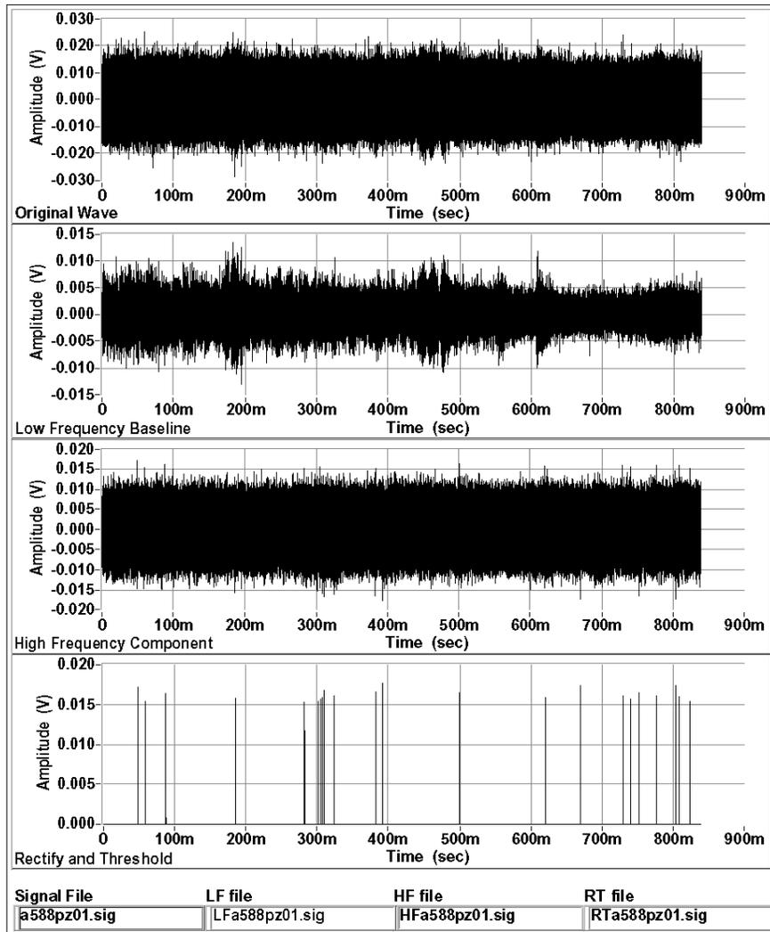
Figure 8. A typical image of AE activity for an A588 sample
