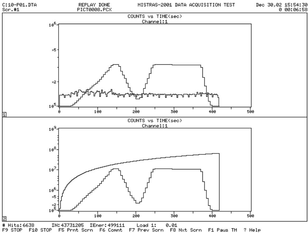
Figure 11 (top) AE activity versus time and Summation of AE versus time, with Load versus time superimposed for thick specimen 10 (base metal); full-scale load corresponds to 2000 lb (bottom) AE activity versus time and Summation of AE versus time, with Load versus time superimposed for thick specimen 10 after plating; full-scale load corresponds to 2000 lb.
