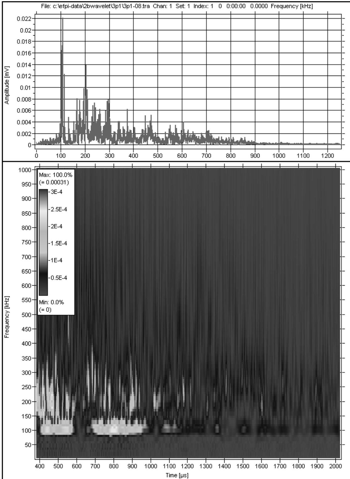
Figure 24. (top) Fast-Fourier Transform (FFT) amplitude versus frequency plot for an AE signal detected during the initial loading of a thin HPS70W specimen 3 after plating, (bottom) Wavelet Transform, frequency versus time.
