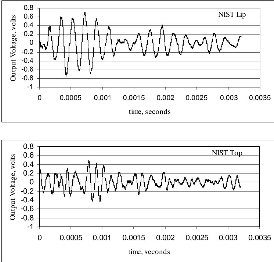
Figure 5. a) Output voltage versus time due to a pencil lead break near the notch tip for a NIST pointducer located on the lip, b) Output voltage versus time due to a pencil lead break near the notch tip for a NIST pointducer located on the top (see Figure 3).
