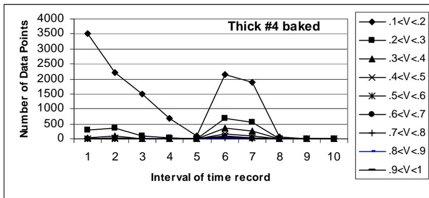
Figure 16. Family of curves showing the distribution of amplitudes over the loading period for thick specimen 4, baked for 2 hours at 400°F.
