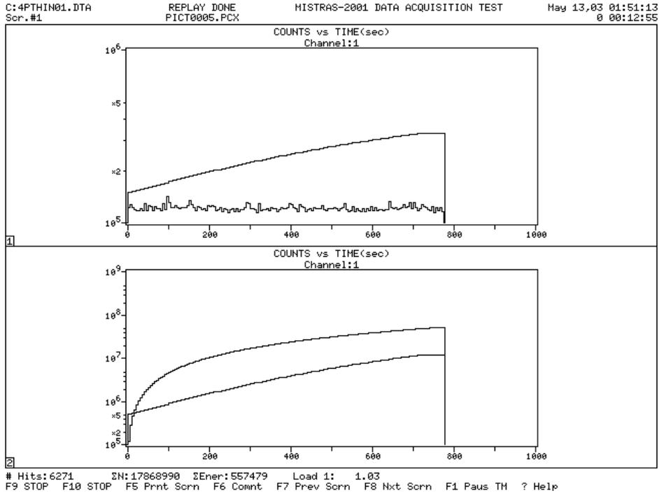
Figure 21b. Plots showing 1) the AE counts versus time and 2) the summation of AE counts versus time during reloading following Zn plating. Superimposed on both plots is the load versus time, where full scale represents 2000 lb.
