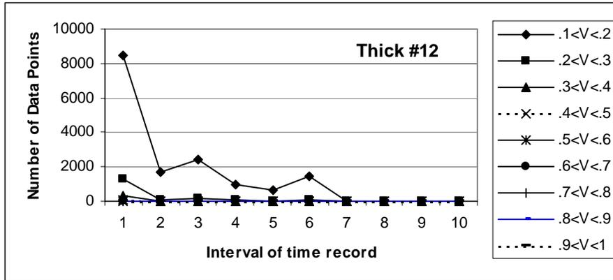
Figure 17. Family of curves showing the distribution of amplitudes over the loading period for thick specimen 12.
