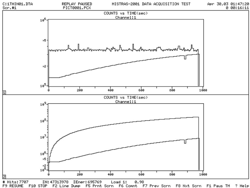
Figure 20a. Plots showing 1) the AE counts versus time and 2) the summation of AE counts versus time during the initial loading. Superimposed on both plots is the load versus time, where full scale represents 2000 lb.
