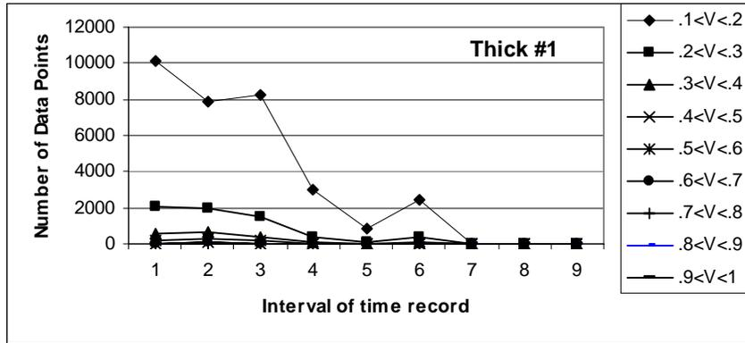
Figure 14. Family of curves showing the distribution of amplitudes over the loading period for thick specimen 1.
