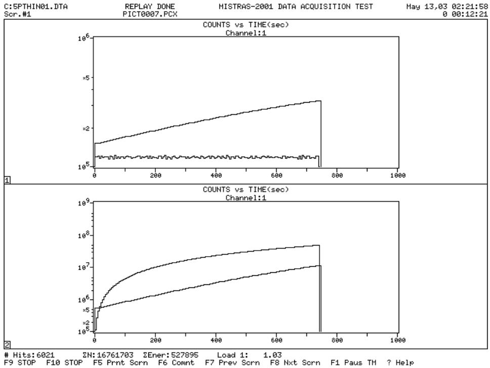
Figure 22b. Plots showing 1) the AE counts versus time and 2) the summation of AE counts versus time during the reloading following Zn plating. Superimposed on both plots is the load versus time, where full scale represents 2000 lb.
