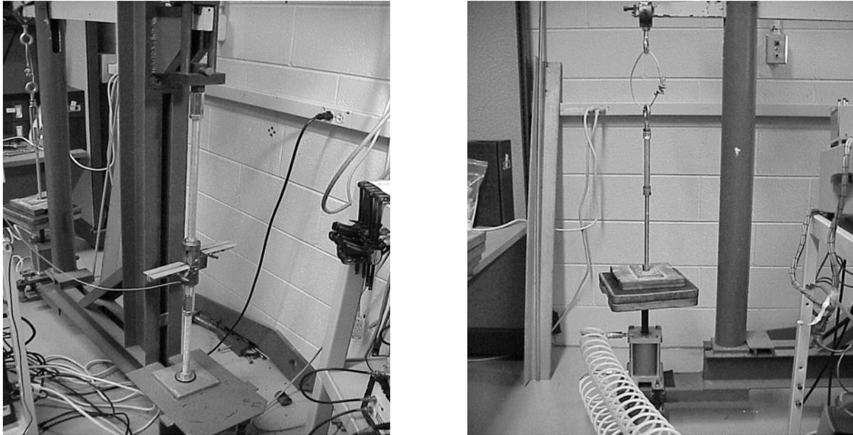
Figure 1. Pictures of the modified dead weight loading system: in the foreground of the image on the left, the specimen gripping fixture can be seen. In the image on the right, the lower portion of the hydraulic weight support unit can be seen beneath some dead weights.
