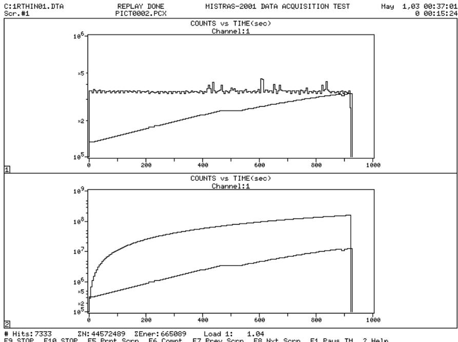
Figure 20b. Plots showing 1) the AE counts versus time and 2) the summation of AE counts versus time during a reloading following Zn plating. Superimposed on both plots is the load versus time, where full scale represents 2000 lb.
