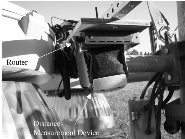
**Figure 14. Router and Distance Measurement Device**
