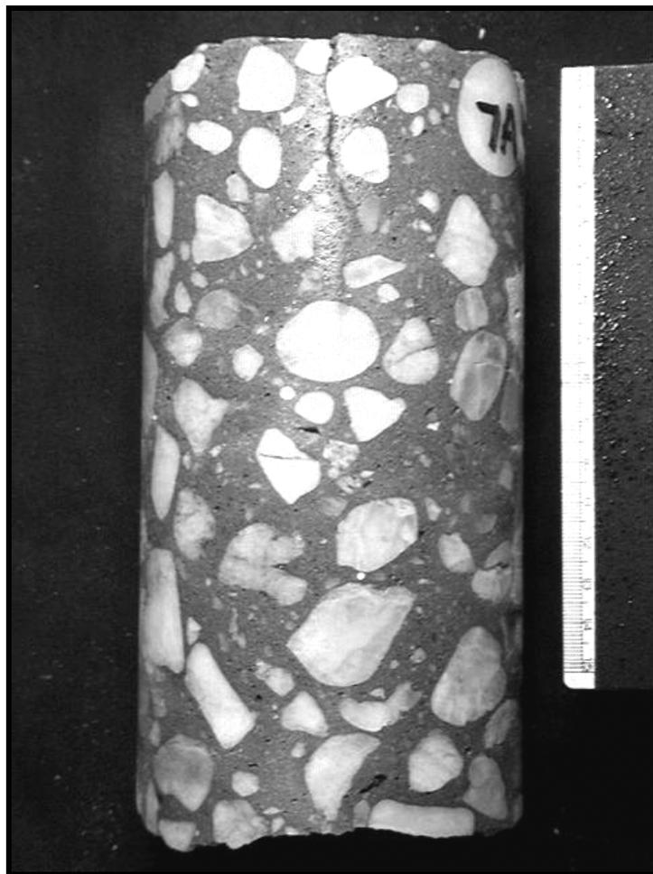
**Figure 14. Core showing crack from surface extending to depth of approximately 2 in where it connects with sub-horizontal network of cracks associated with coarse aggregate particles.**
