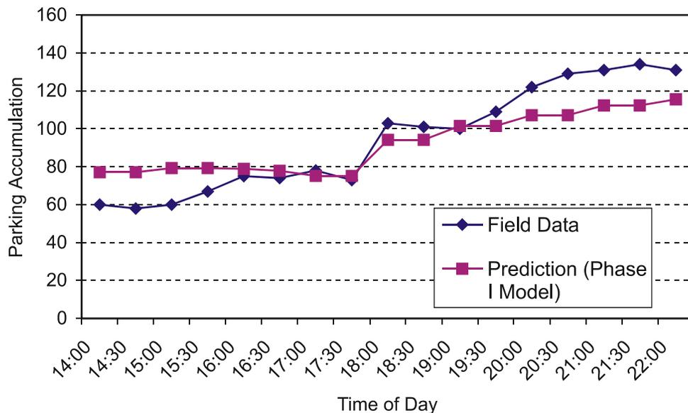
Figure 9. Estimated Parking Accumulation from Model vs. Field Data at Ashland Travel Center
