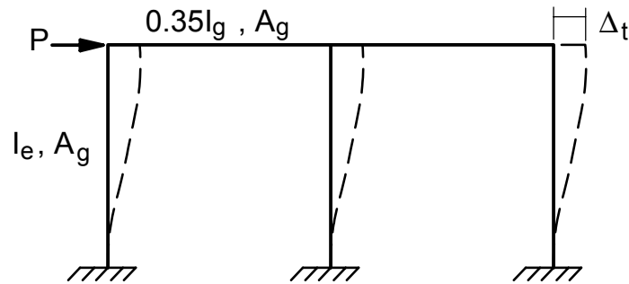
Figure 33. The loading to the substructure to determine the stiffness in the transverse direction.
