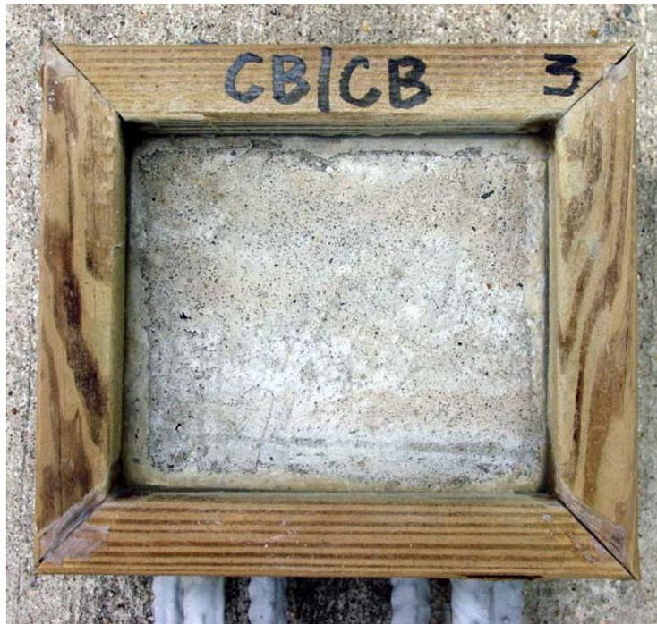
**Figure 15. Top View of Concrete Block With Clad Bars at Top And Bottom With No Sign of Corrosion, Even After 700 Days.** Blocks with stainless steel bars were similarly free of corrosion.
