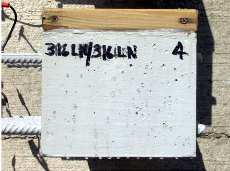
**Figure 24. Side View of Concrete Block With 316LN Stainless Steel Bars at Both Top and Bottom.** No sign of corrosion is present, even after 650 days of severe weekly cycles of salt ponding and drying.
