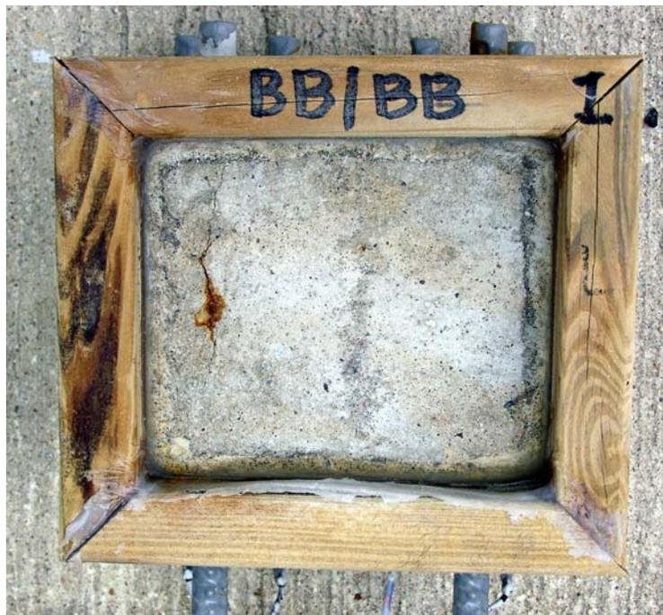
**Figure 14. Top View of CS/CS (BB/BB) Concrete Block Showing Severe Corrosion of Top Carbon Steel Bar and Resulting Concrete Damage, After 700 Days.**
