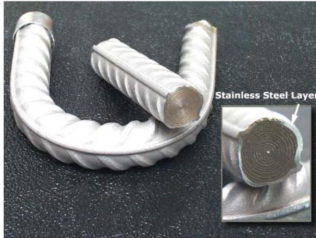
**Figure 1. Stainless Steel–Clad Bars Obtained From Stelax UK Limited, West Glamorgan, U.K.**
