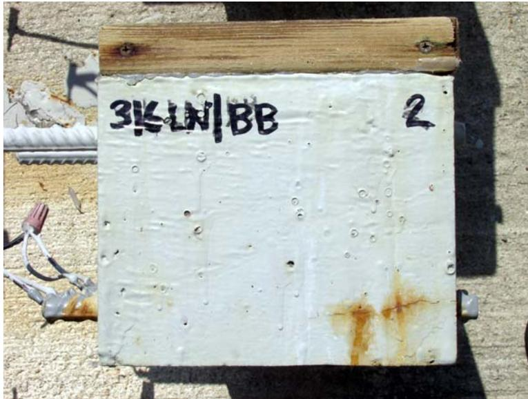
**Figure 23. Side View of Concrete Block With 316LN Stainless Steel Bars at Top and Carbon Steel Bars at Bottom.** Notice the rust stain and cracking at the lower right corner attributable to corrosion on the bottom carbon steel bars.
