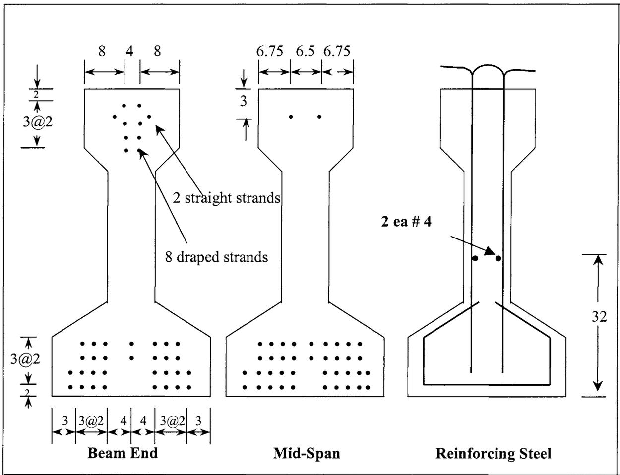
**Figure 6: Non-Composite Type IV Prestressed Test Girders**
