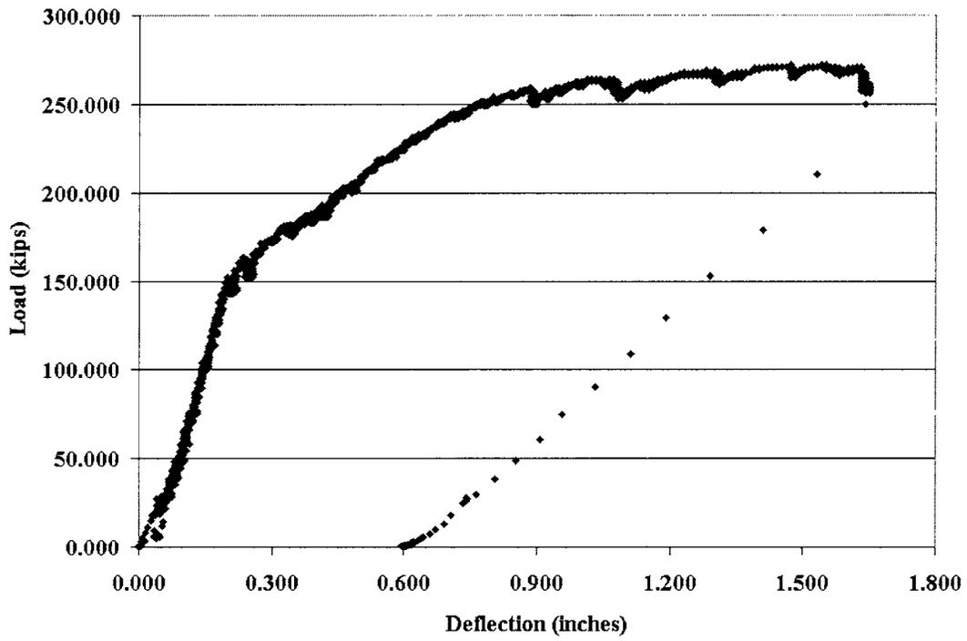
**Figure 12: Load Deflection Curve: Beam LW8000II-2C-72**
