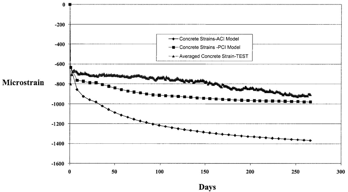
**Figure 17: Variation of Concrete Strains vs. Time**
