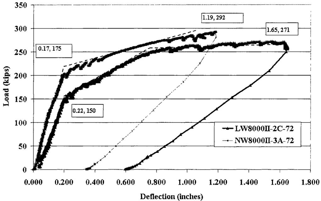
Figure 14: Typical Load Deflection Curve for HPLWC/HPNWC Beams
