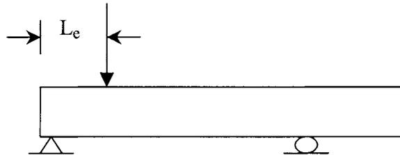
**Figure 4: Development Length and Flexural Strength Testing Scheme**
