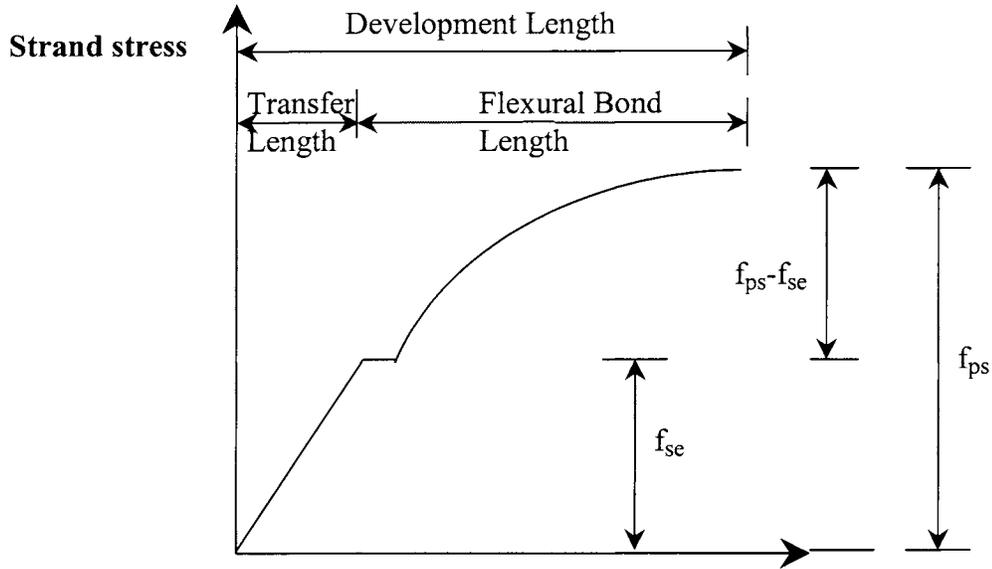
**Figure 3: Variation of Steel Stress with Distance from Free End of Strand<sup>6</sup>**
