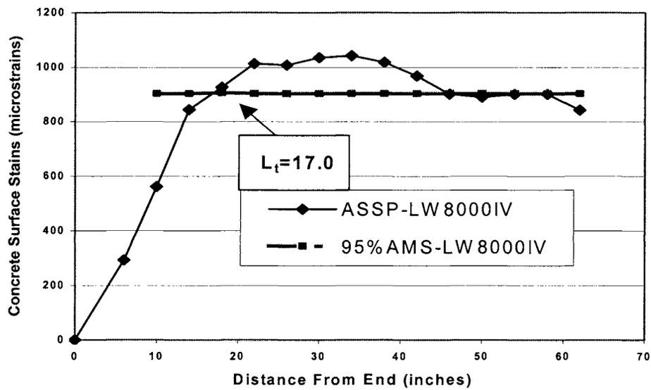
Figure 10: Averaged Strain Profile for Both HPLWC Type IV Test Beams
