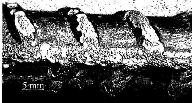
Figure 12. Visual appearance of carbon steel rebar repassivation specimen after potential step down test, conducted in sand-glass beads with saturated  $\text{Ca}(\text{OH})_2 + 0.1 \text{ M NaCl}$  solution ( $\text{Cl}^-/\text{OH}^- = 4$ ).
