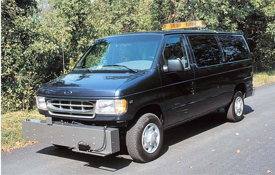
**Figure 3. Inertial Profiler**
