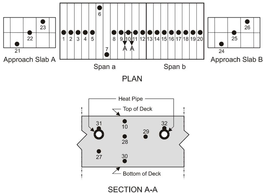
Figure 6. Layout of Temperature Monitoring Probes
