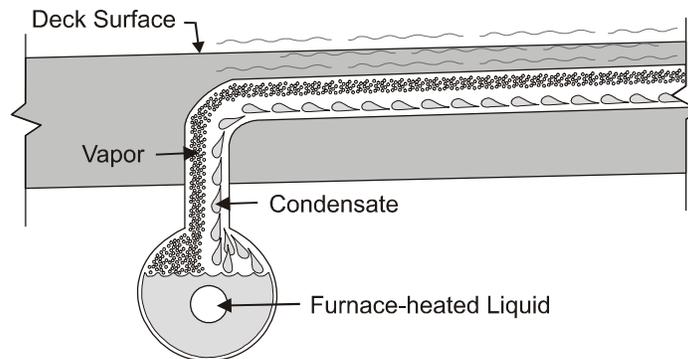
**Figure 3. Cross Section of Heating Element**
