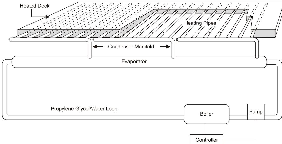
**Figure 2. Schematic of Heat Pipe System**
