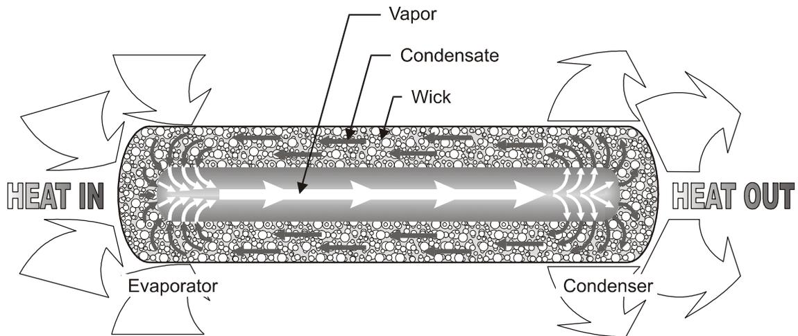
**Figure 1. Heat Pipe Principle**
