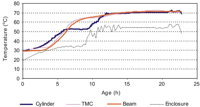
**Figure 27. Temperature Development in Bridge Beam**
