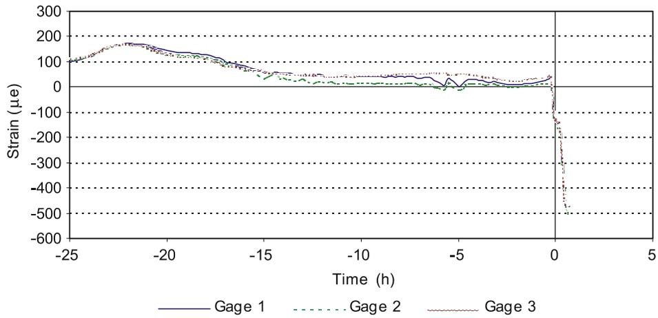
**Figure 33. Strain Versus Time for Beam 2**
