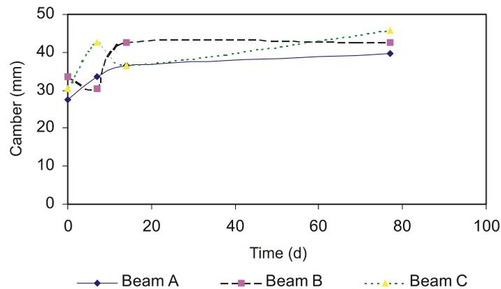
**Figure 35. Midspan Camber Versus Time**
