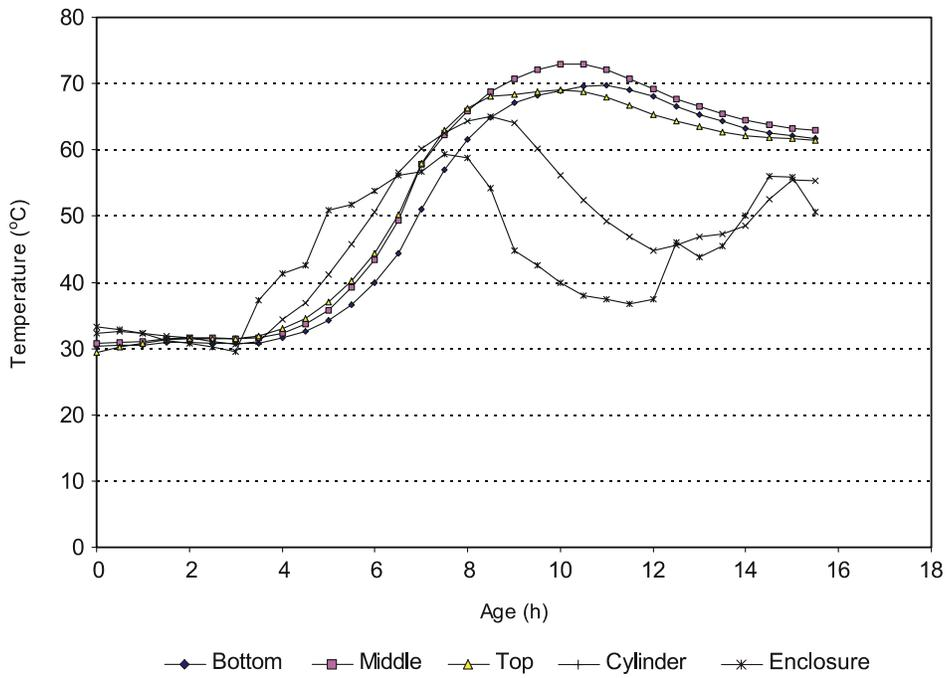
**Figure 6. Temperature Development in Test Beam 2**
