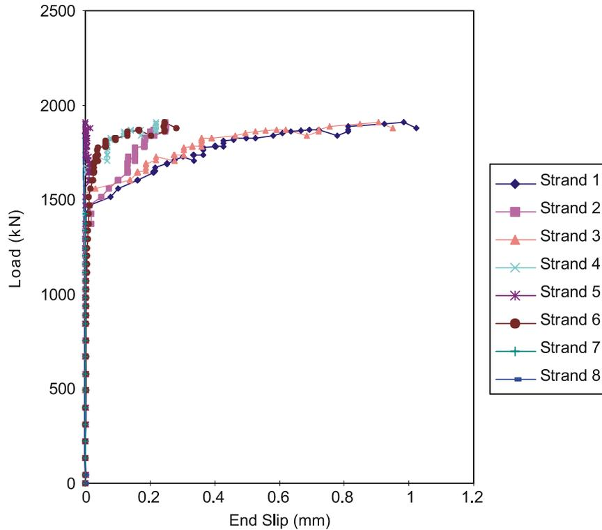
**Figure 21. End Slip Versus Load for Test Beam 2, End B**
