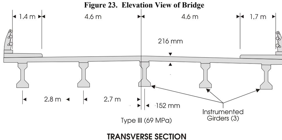
**Figure 24. Transverse Section of New Bridge Showing Location of Instrumented Beams**
