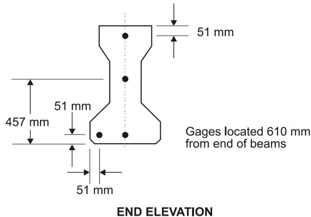
**Figure 3. Location of Temperature Gages in Test Beams**
