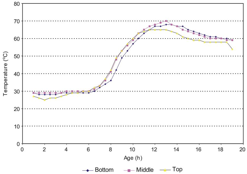
**Figure 5. Temperature Development in Test Beam 1**
