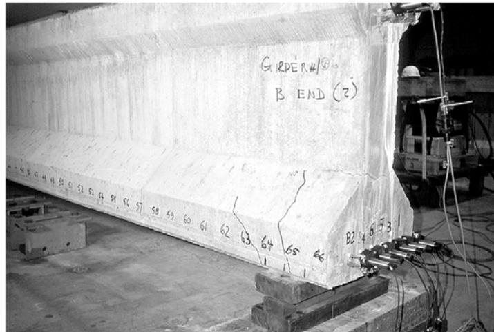
**Figure 4. Measurement of End Slippage by LVDTs**
