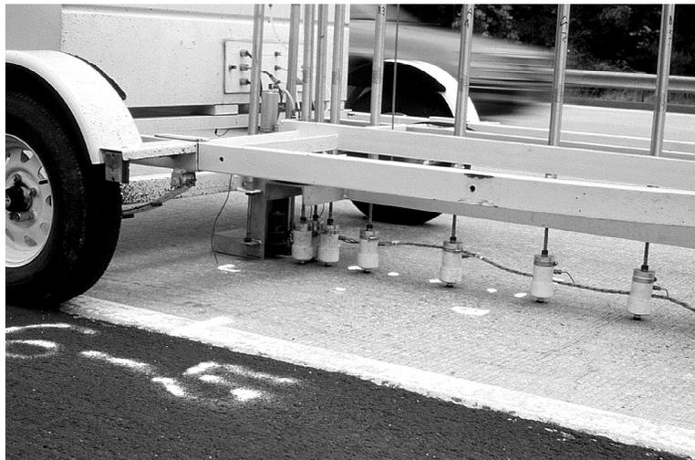
**Figure 9. Trailer-mounted SPA, equipped with two pneumatic hammers and several transducers, positioned over test location.**
