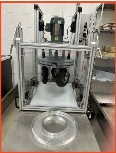
The three-wheel polishing device is used for friction testing in the asphalt lab.
