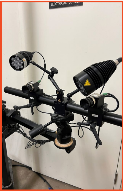
The digital image correlation system can help determine the stress capacity of steel beams for bridges and other infrastructure.
